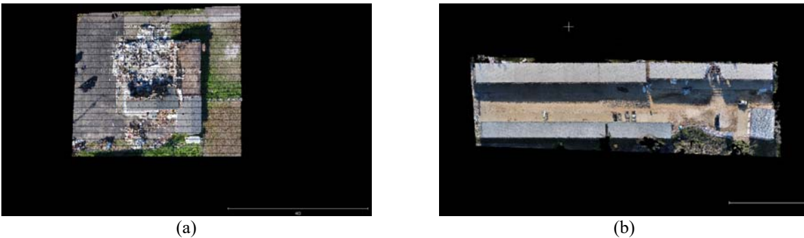
Figure 2. SfM derived point clouds: (a) VFW and (b) Aransas Pass storage facility
