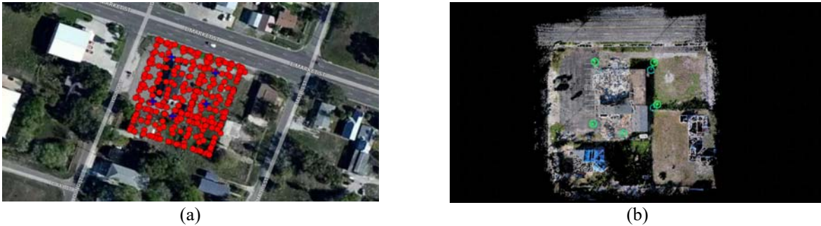
Figure 1. VFW flight details: (a) image locations in red and (b) GCPs shown in green
