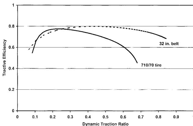
Figure 2—Tractive efficiency vs dynamic traction ratio for the 81-cm (32-in.) belt and 710/70 rear tires on a non-tilled wheat stubble field.
