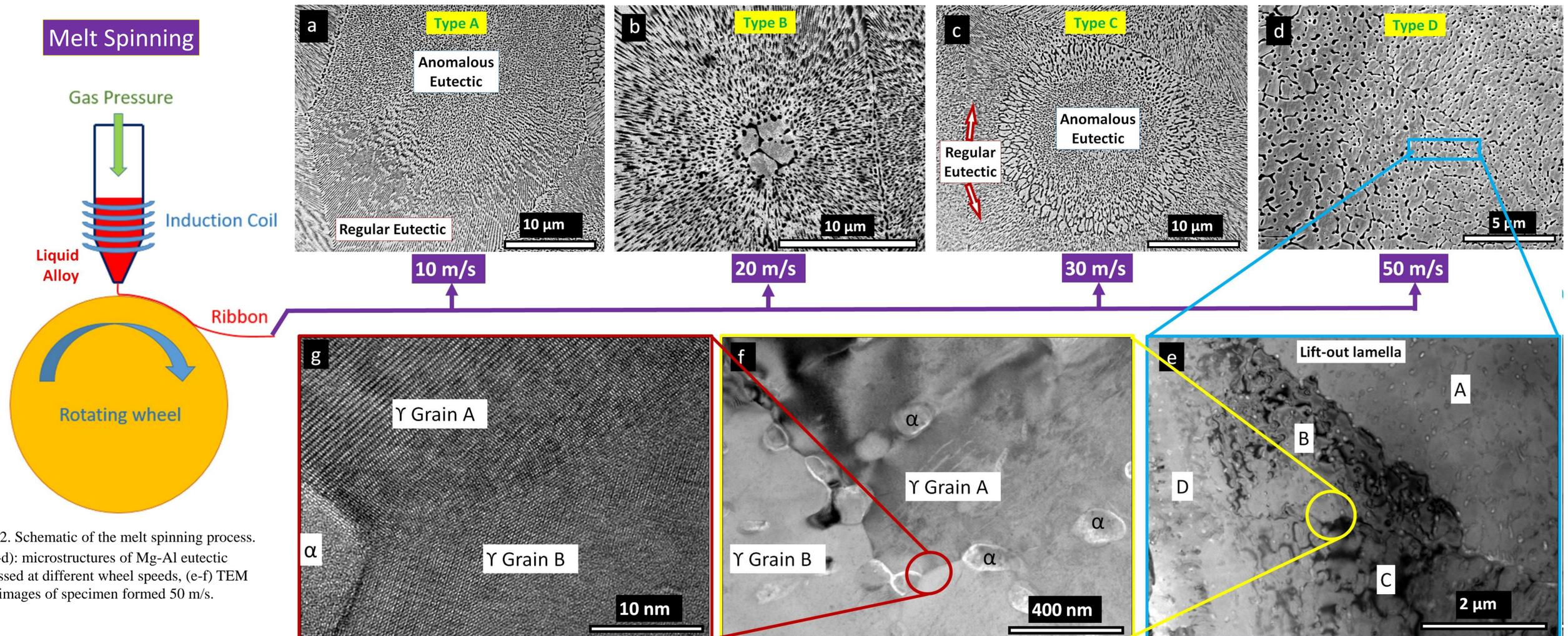
Figure 2. Schematic of the melt spinning process. (a-d): microstructures of Mg-Al eutectic processed at different wheel speeds, (e-f) TEM images of specimen formed 50 m/s.
