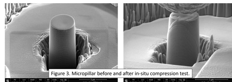
Figure 3. Micropillar before and after in-situ compression test.
