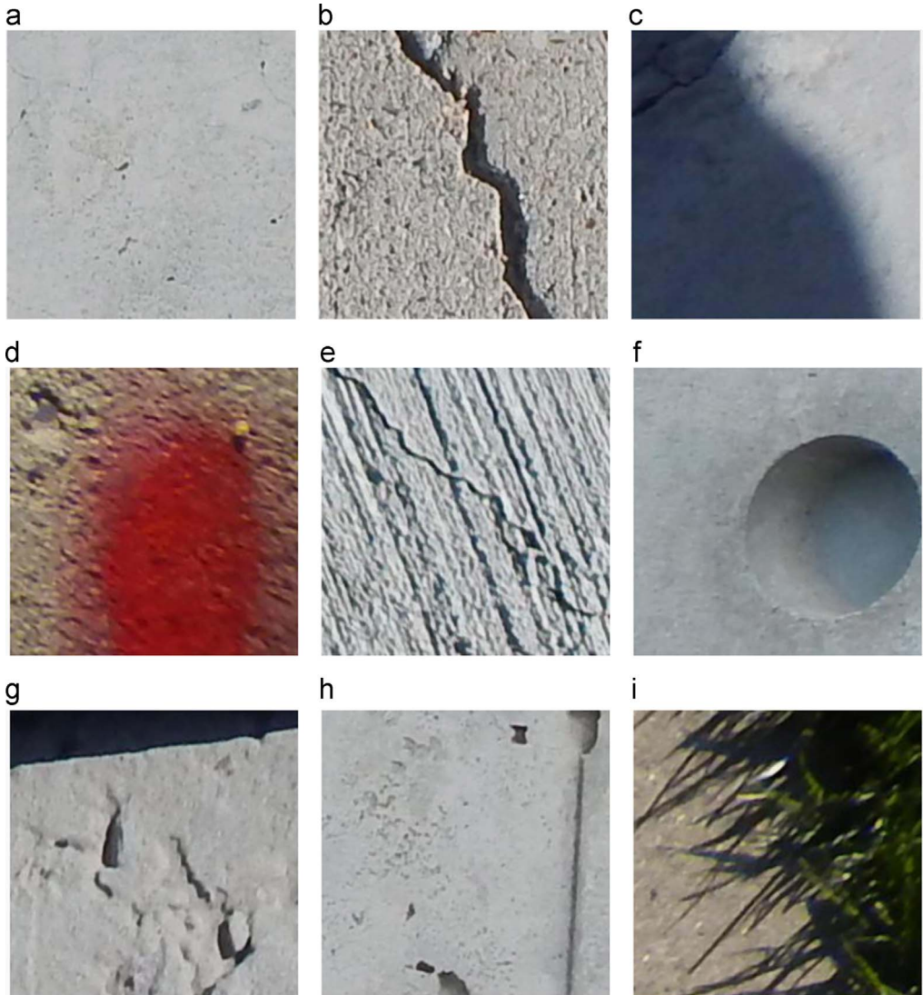
Fig. 1. SDNET2018 images include (a) fine cracks, (b) coarse cracks, (c) shadows, (d) stains, (e) rough surface finishes, (f) inclusions and voids, (g) edges, (h) joints and surface scaling, and (i) background obstructions.
