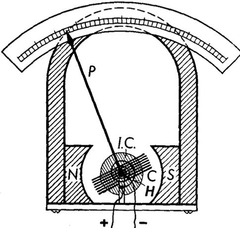
**Fig. 31-11** Essentials of a moving coil galvanometer. *C* is the moving coil, *N* and *S* are the poles of a permanent magnet, *I.C.* is the soft iron core, *P* is the pointer, and *H* is the hairspring.
