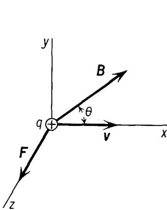
Fig. 31-1 The force  $\mathbf{F}$  exerted on a charge  $q$  moving with velocity  $\mathbf{v}$  in a magnetic field of induction  $\mathbf{B}$ .  $\mathbf{B}$  and  $\mathbf{v}$  are in the  $x$ - $y$  plane;  $\mathbf{F}$  is along the  $z$  axis.
