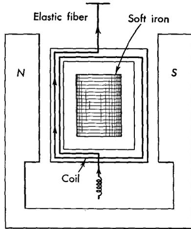
**Fig. 31-10** Essentials of a D'Arsonval type of galvanometer. The soft iron core is introduced to shape the magnetic field so that it is radial, thus obtaining a galvanometer in which the deflection is proportional to the current through the coil.
