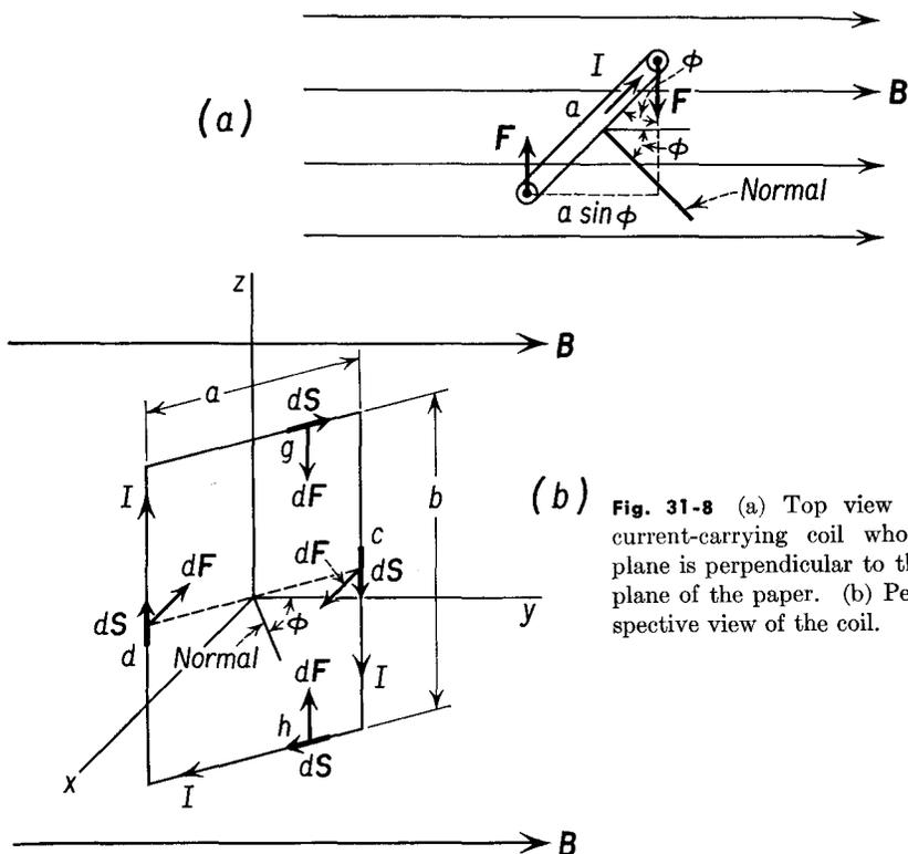
Fig. 31-8 (a) Top view of current-carrying coil whose plane is perpendicular to the plane of the paper. (b) Perspective view of the coil.
