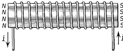
Fig. 33-1 A solenoid containing a ferromagnetic core.
