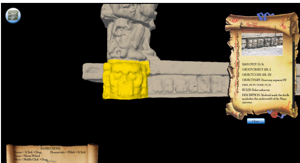
Figure 16: Example of a query on a single segmented object at LoD4: information regarding the segmented architectural elements of the interior doorframe is shown.
