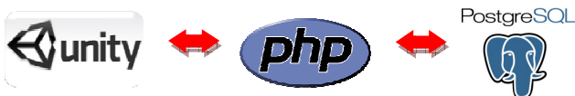
Figure 5: Schematic representation of the data exchange between Unity and PostgreSQL, using PHP as interface.
