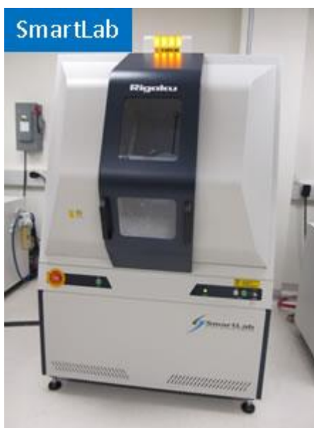
Figure 2.5: Rigaku SmartLab Diffractometer in a laboratory setting, used for detailed crystallographic analysis of materials
