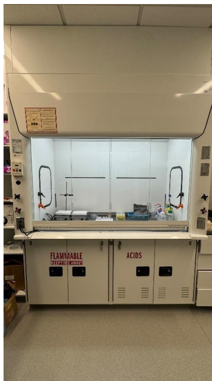
Figure 2.1: A fume hood in a laboratory setting, equipped for safely handling and venting hazardous chemicals, ensuring a controlled environment for experiments involving flammable and acidic substances.
