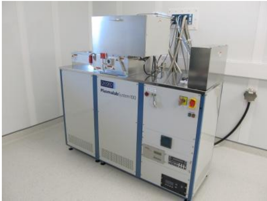
Figure 2.4: Oxford PlasmaPro 100 Deep RIE System in a cleanroom environment, used for precise etching of semiconductor materials.
