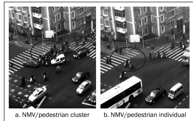
Figure 1 - The process of NMVs/pedestrians entering the intersection
