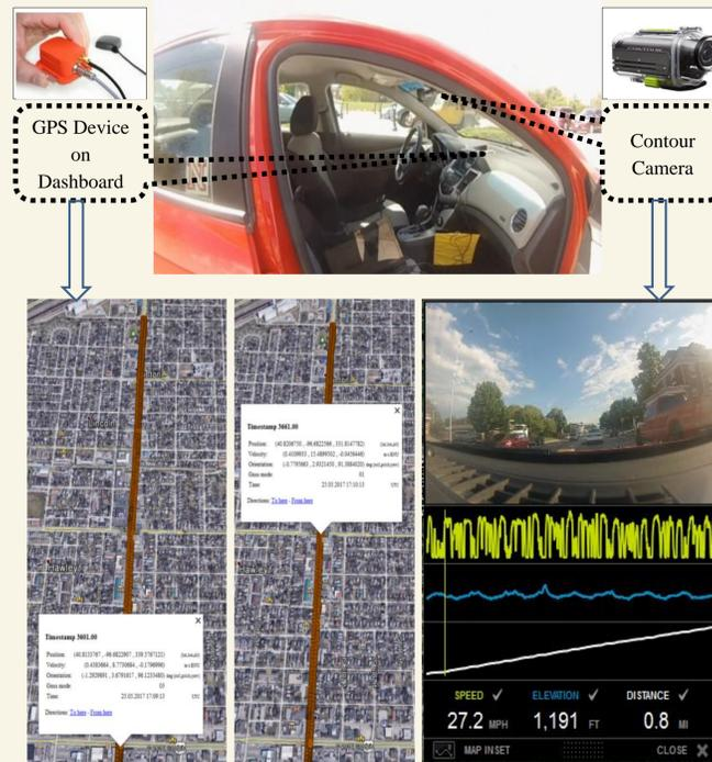
Figure 3: Test vehicle setup showing (a) GPS trajectory with time stamps, and (b) speed profiles
