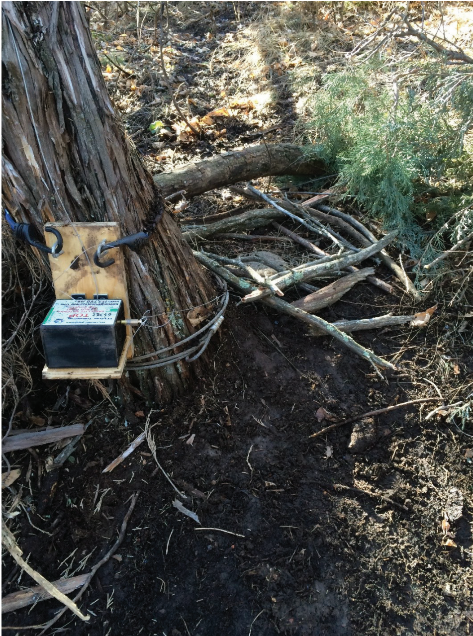
Figure 2. Example of the typical setup used to monitor foothold traps set to capture mountain lions in the North Dakota Badlands from 2014–2016. The TT3 and bracket was attached to the base of the trap tree with a bungee cord. The trap (inside the rectangle of guiding sticks) was attached to a cable wrapped tightly around the base of the tree. Finally, the trigger pin was attached to the trap chain with a steel fishing leader.
