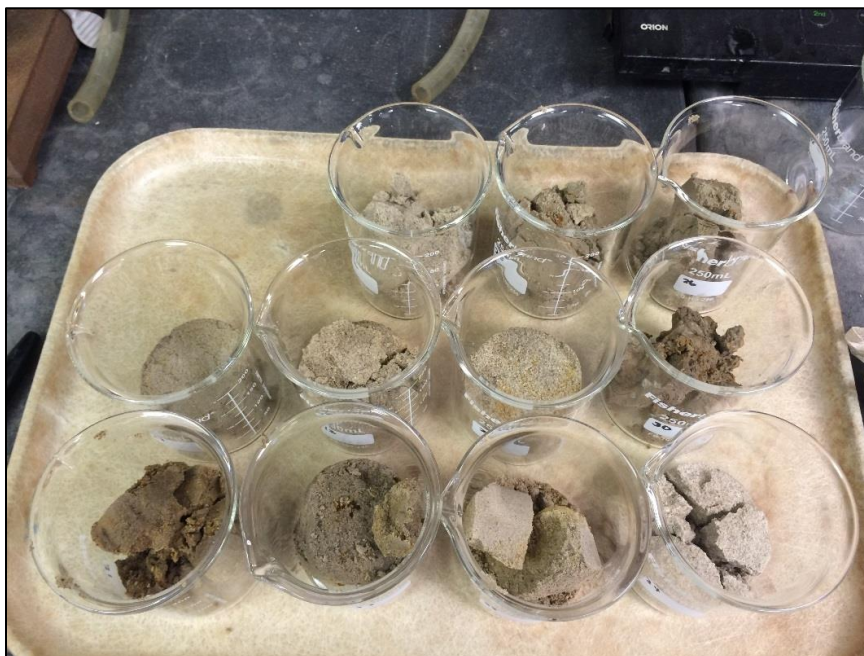
Figure 11: Segments of core aliquots after being dried overnight for bulk density and moisture content analysis.
