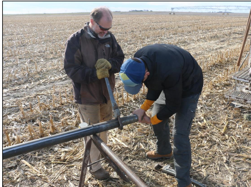
Figure 10: Extruding a core liner from a CME drill's hollow stem auger at HC-11-W.
