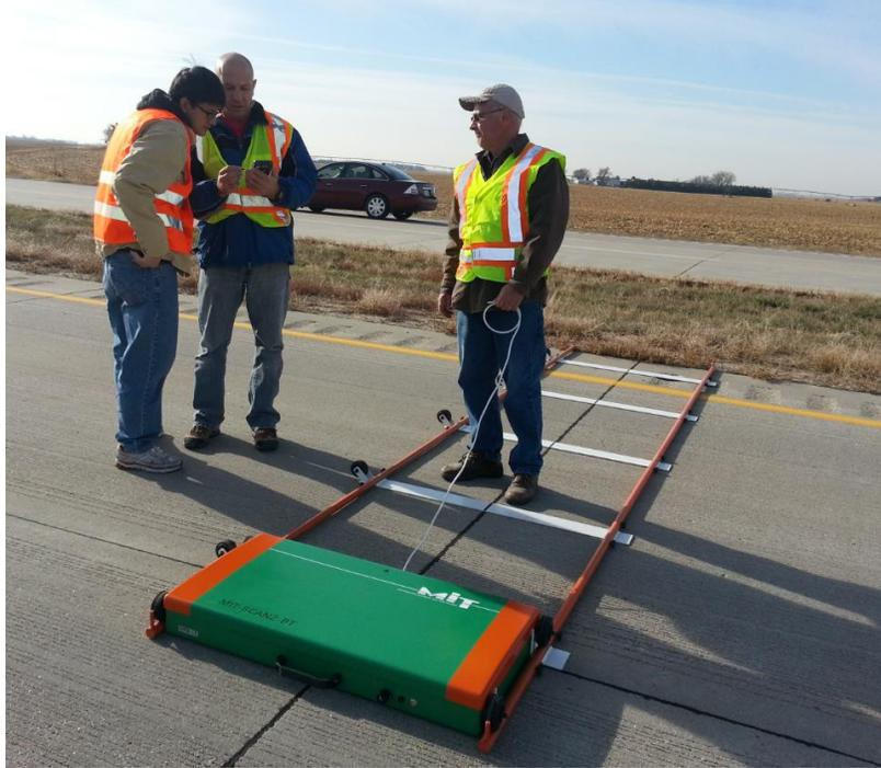
**Figure 1.3** A joint being scanned by MIT Scan-2
