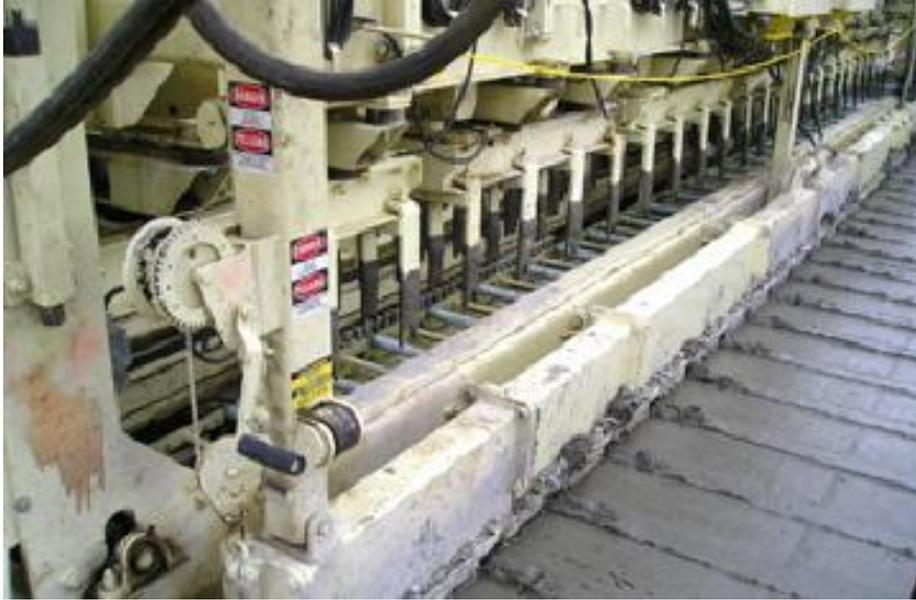
**Figure 1.2** Dowel Bar Inserter (DBI)
