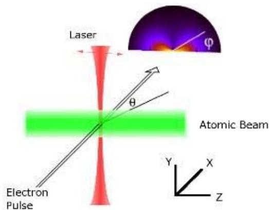
An illustration of an experiment modeled by Hua-Chieh Shao and Anthony Starace. It shows the 110-attosecond electron pulse sent through a beam of hydrogen atoms (green) excited by a laser (red). The distribution pattern of the scattered electrons is in the background.
