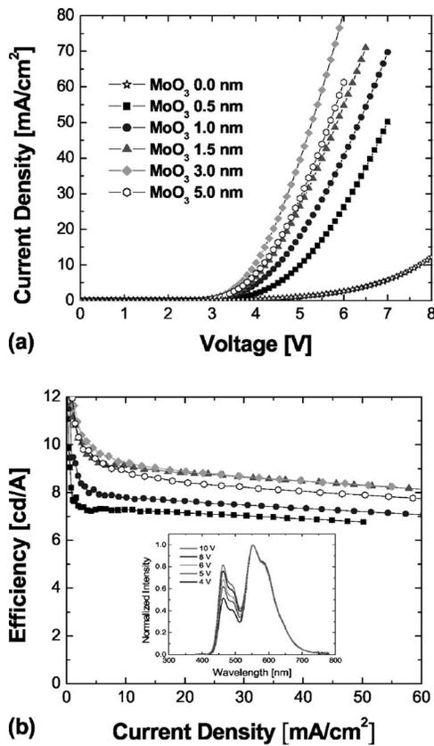
FIG. 2. (a)  $J$ - $V$  characteristics and (b) efficiency as a function of current density for top-emission devices with different  $\text{MoO}_3$  thicknesses. The structure of top-emitting PLEDs:  $\text{Al}(100 \text{ nm})/\text{MoO}_3(X \text{ nm})/\text{PEDOT:PSS}(25 \text{ nm})/\text{LEP}(80 \text{ nm})/\text{Cs}_2\text{CO}_3/\text{Ca}(10 \text{ nm})/\text{Ag}(10 \text{ nm})$ ,  $X$  from 0 to 120 nm. The inset of (b) shows EL spectra of devices under different biases.
