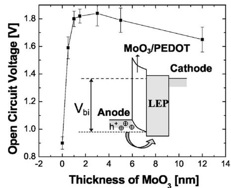
FIG. 3. Open circuit voltage as a function of  $\text{MoO}_3$  thickness. The inset shows a schematic diagram to explain the reduction of barrier height for hole injection with a  $\text{MoO}_3$  layer in the anode structure.
