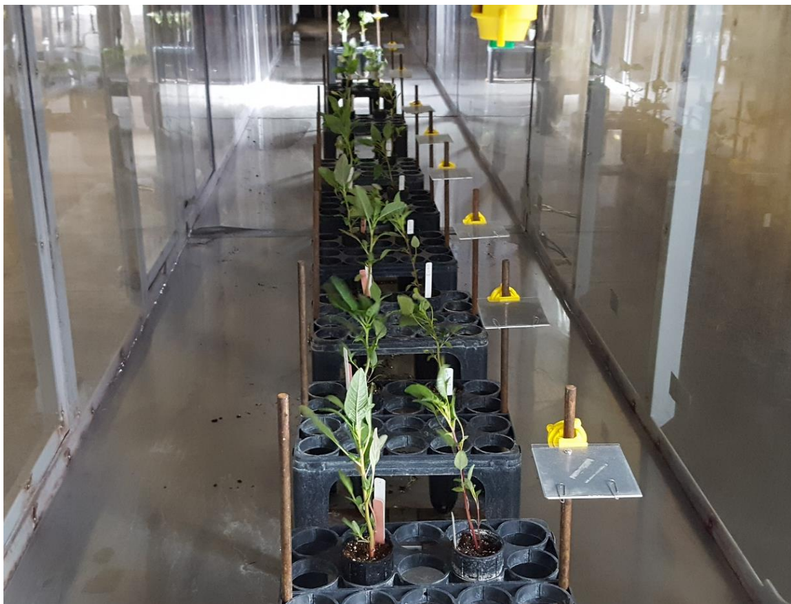
Figure 3.2. Herbicide particle drift study conducted in the low speed wind tunnel with waterhemp ( Amaranthus tuberculatus ), Palmer amaranth ( Amaranthus palmeri ), and drift collectors (Mylar cards) positioned at different downwind distances from the nozzle.
