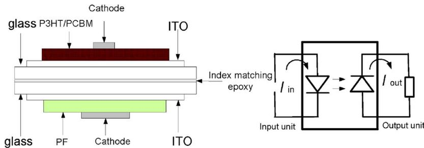
FIG. 1. (Color online) Schematic structure and corresponding circuit of the optocoupler.
