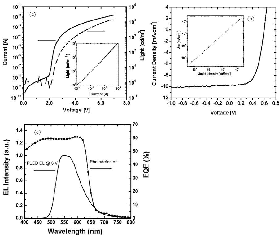
FIG. 2. (a) Current-luminance-voltage characteristic of PLED. Inset: luminance vs current. (b)  $J$ - $V$  characteristic of the photodiode under AM1.5G 100 mW/cm<sup>2</sup> illumination. Inset: short-circuit current density ( $J_{sc}$ ) dependence on the incident light intensity. (c) EL spectrum of PLED and EQE for the photodiode.
