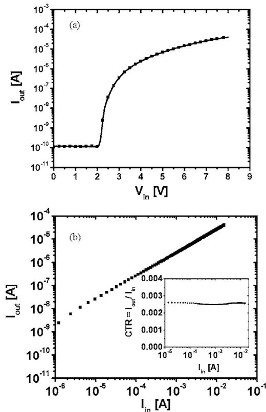
FIG. 3. (a) Current of the photodiode ( $I_{out}$ ) vs voltage of the PLED ( $V_{in}$ ) with photodiode under no bias condition. (b) Current transfer characteristics: current of the photodiode ( $I_{out}$ ) vs current of the PLED ( $I_{in}$ ). Inset: current transfer ratio vs  $I_{in}$ .
