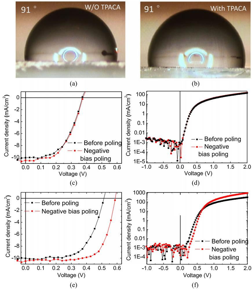
Fig. 3. Contact angle measurement of the PHT:PC<sub>60</sub>BM film (a) without and (b) with TPACA blended in the active layer. (c) Photocurrent and (d) dark current of the device before and after negative bias poling after methanol washing with TPACA as interfacial layer. (e) Photocurrent and (f) dark current of the device before and after negative bias poling after methanol washing with TPACA blended in the P3HT:PC<sub>60</sub>BM active layer.
