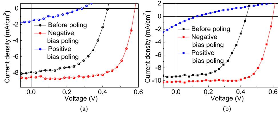
Fig. 2. (a) Photocurrent of the P3HT:PC<sub>60</sub>BM device before and after negative bias poling with TPACA as cathode interfacial layer. (b) Photocurrent of the P3HT:PC<sub>60</sub>BM device before and after poling with TPACA blended in the active layer.
