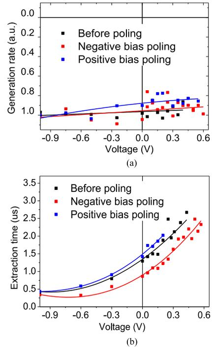
Fig. 5. (a) Charge generation rate measured by time delayed collection field. The charge generation efficiencies were measured under different bias from  $-4$  V to open-circuit voltage and were normalized by the internal quantum efficiency at  $-4$  V. (b) Charge extraction time of the device before and after poling.
