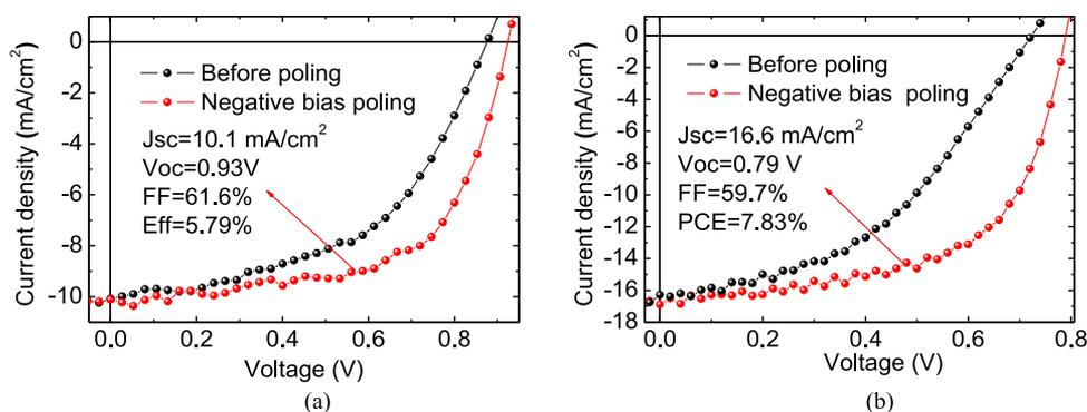
Fig. 6. TPACA polar molecule application in (a) PCDTBT:PC<sub>70</sub>BM system and (b) PBDTTT-CT:PC<sub>70</sub>BM system with TPACA blended in the active layer.
