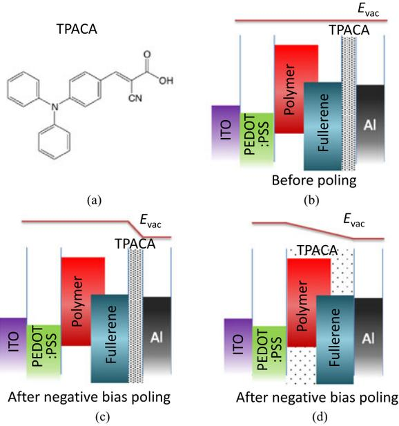
Fig. 1. (a) Molecular structure of TPACA. Energy diagram of the device (b) before poling and (c) after negative bias poling with TPACA as the cathode interfacial layer. (d) Energy diagram of the device after negative bias poling with TPACA blend in the active layer.
