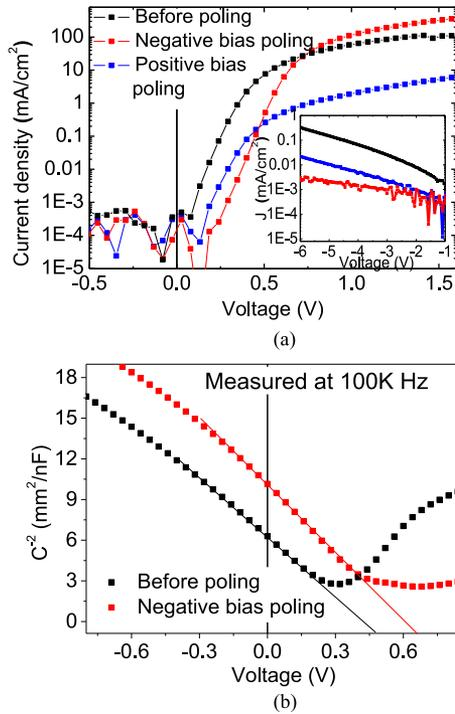
Fig. 4. (a) Dark current of the device with TPACA blended in the active layer. The inset is the dark current of the device under negative bias. (b) Built-in potential of the P3HT:PC<sub>60</sub>BM device measured by fitting the  $1/C^2$  versus voltage curve.
