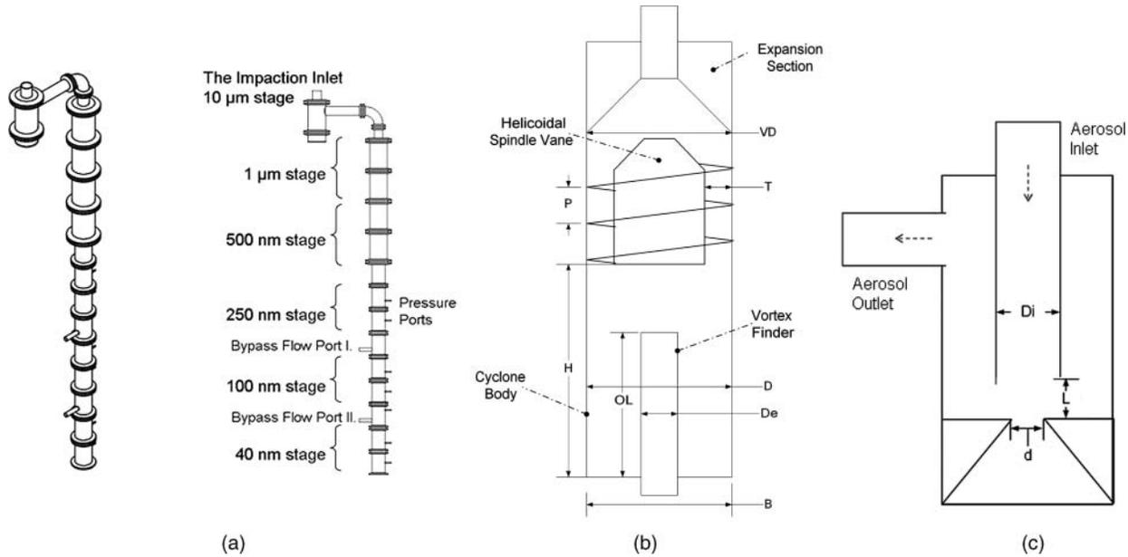
FIG. 1. (a) Schematic diagram of the overall system of the prototype. (b) Schematic diagram of an axial flow cyclone stage (Stages #1–5). (c) Schematic diagram of the impaction inlet.
