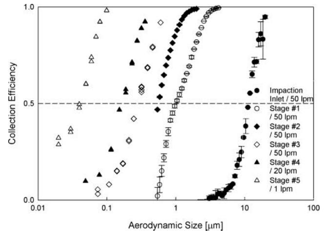
FIG. 4. Measured collection efficiency curves of the impaction inlet and individual cyclone stages of the prototype.
