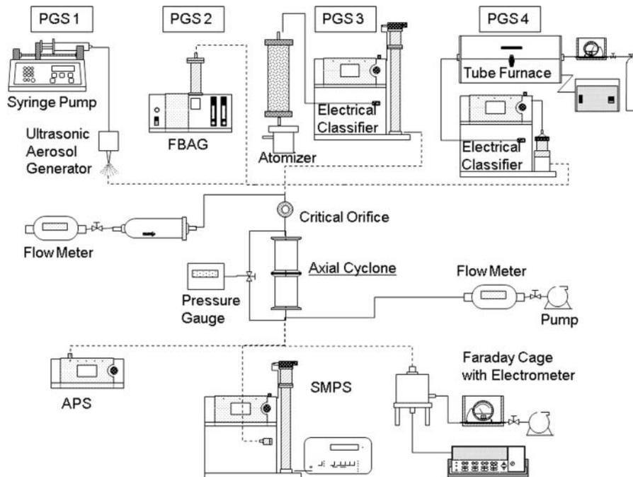
FIG. 2. Schematic diagram of experimental setup for the calibration of the impaction inlet and individual cyclone stages.
