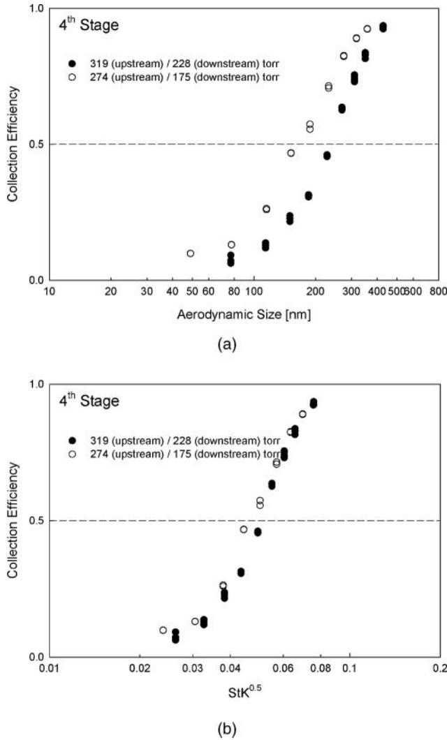
FIG. 3. Particle collection efficiency curves for the 4th cyclone stage under two different pressure conditions (i.e., 319 torr and 274 torr) at 20 lpm. (a) aerodynamic size as the abscissa; (b) square root of  $StK$  number as the abscissa.
