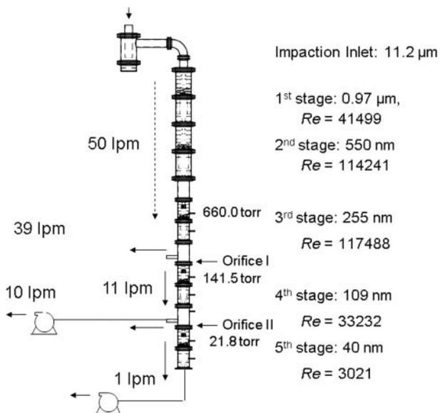
FIG. 7. Overall flow operation scheme of the prototype and the corresponding cutoff sizes for the impaction inlet and cyclone stages.
