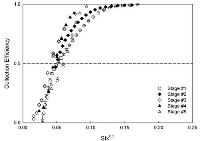
FIG. 5. Collection efficiency curves as a function of the particle Stokes number for all the axial flow cyclone stages of the prototype.
