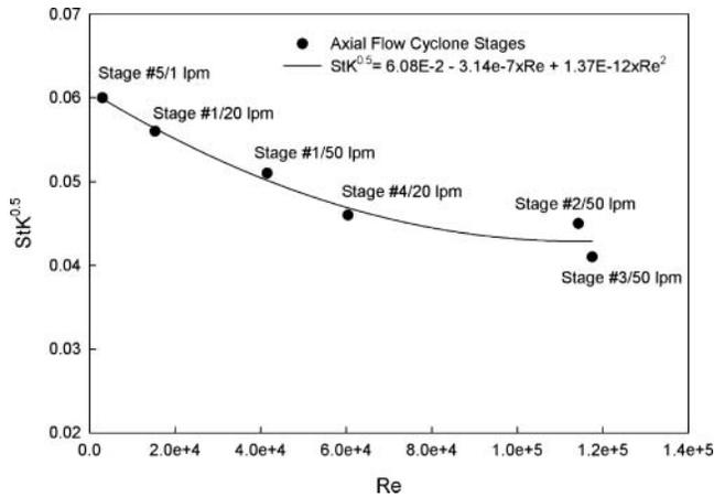
FIG. 6. Dimensionless cutoff size ( $StK_{50}^{0.5}$ ) vs. flow Reynolds number for all axial flow cyclone stages.
