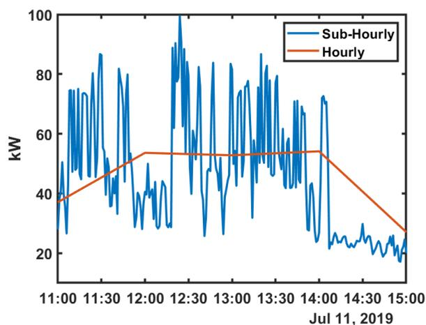
FIGURE 3. One-minute measurements and aggregated hourly measurements for an actual building on July 11, 2019.
