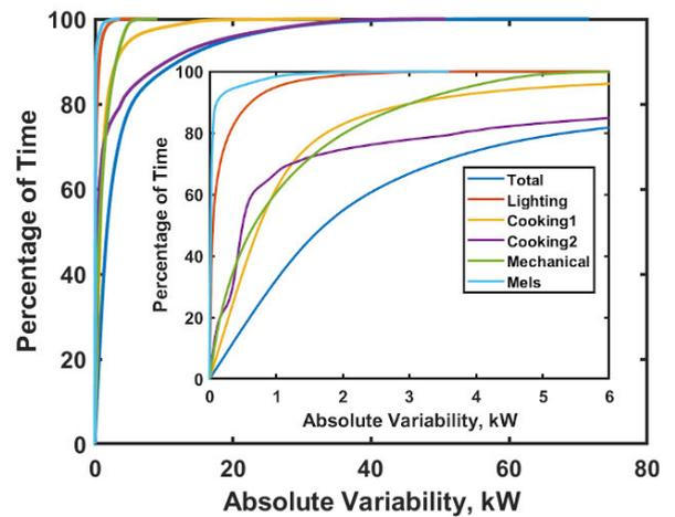
FIGURE 16. Cumulative distribution of absolute variability for the full building and all end-use load categories, over a full year. The inlaid plot zooms in on the leftmost portion of the distribution.
