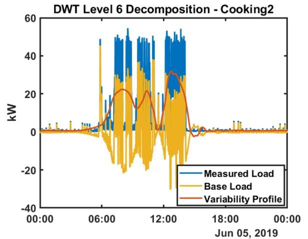
a) Result of applying a DWT level 6 decomposition on a sample daily Cooking2 load profile.
