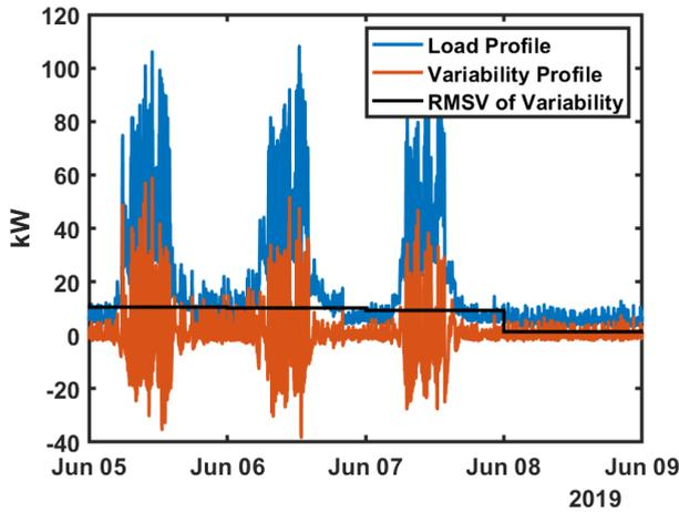
FIGURE 17. Full building load profile and variability for 4 days, with RMSV.
