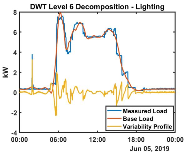
FIGURE 12. Sample daily Lighting category profile, with extracted base load and variability.
