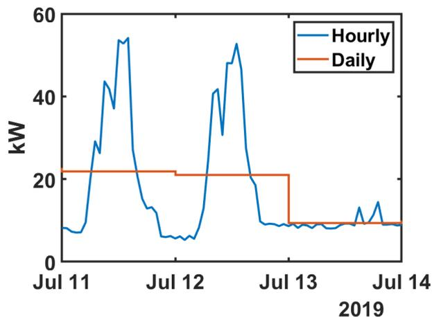
FIGURE 2. Hourly and aggregated daily load profile measurements for an actual building on July 11-14, 2019.
