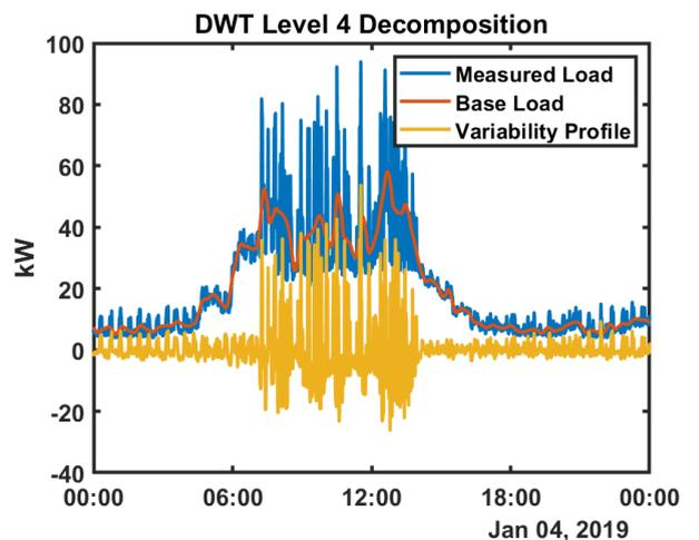
**FIGURE 10.** Result of applying a DWT level 4 decomposition on a sample daily load profile.
