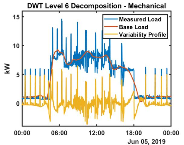
b) Result of applying a DWT level 6 decomposition on a sample daily Mechanical load profile.
