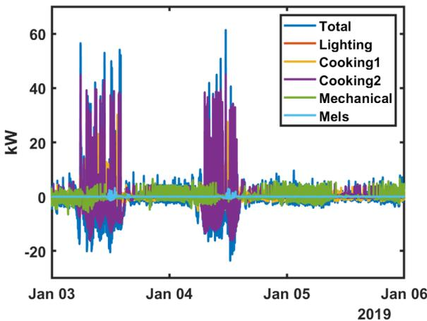
FIGURE 15. Variability profiles for the building's end-use load categories over 3 days.
