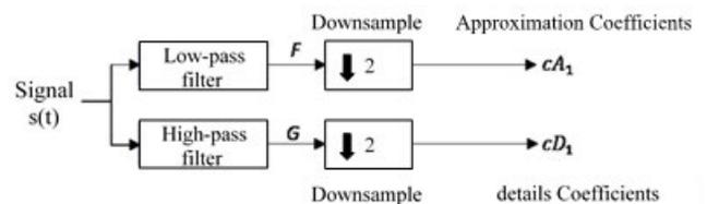
FIGURE 5. 1-level DWT process.
