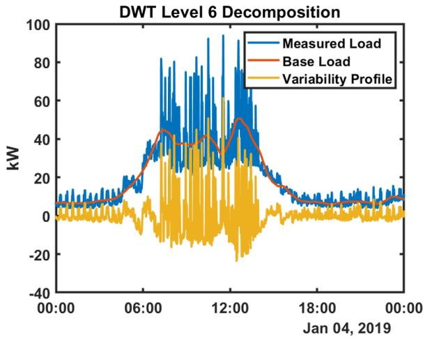
FIGURE 11. Result of applying a DWT level 6 decomposition on a sample daily load profile.
