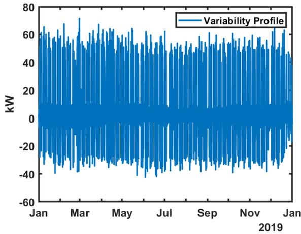
FIGURE 14. Full year Variability profile for the total building load profile.
