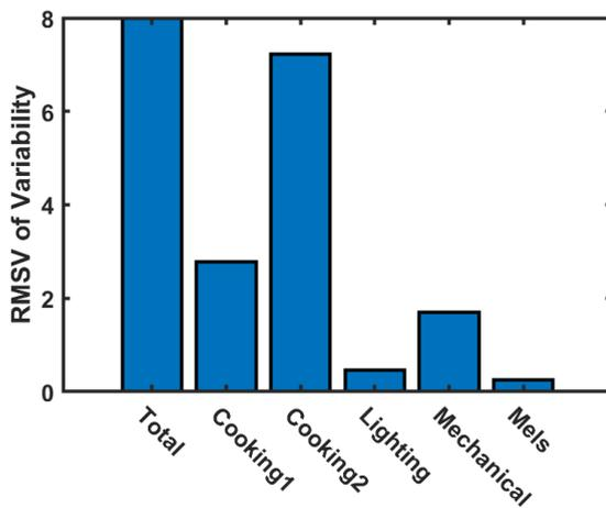
FIGURE 18. Yearly RMSV for the total building and its end-use load categories.
