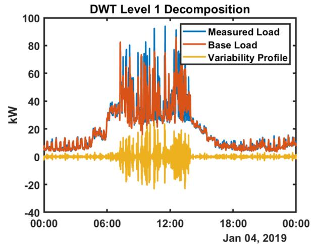
**FIGURE 9.** Result of applying a DWT level 1 decomposition on a sample daily load profile.
