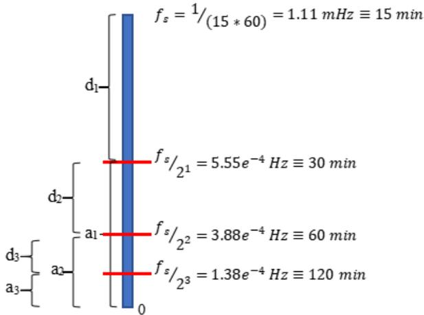
FIGURE 6. DWT - 3 levels of decomposition process.
