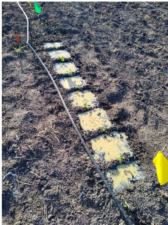
Figure 5. Bio-based sprayable mulch film applied on 27 August 2019 on the East campus research farm at the University of Nebraska-Lincoln. Solution was applied via a graduated cylinder within a 0.09 m 2 area between kale plants at two rates, 4.07 and 6.11 L/m 2 (pictured), prior to the emergence of mustard seedlings.
