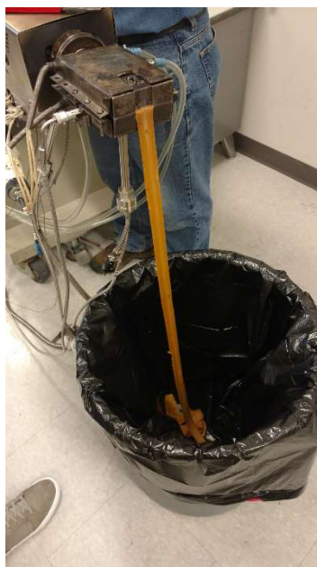
Figure 3. A bio-based formulation is produced from an extruder as a 4 cm wide strip. After the product dries it is ground into a powder.
