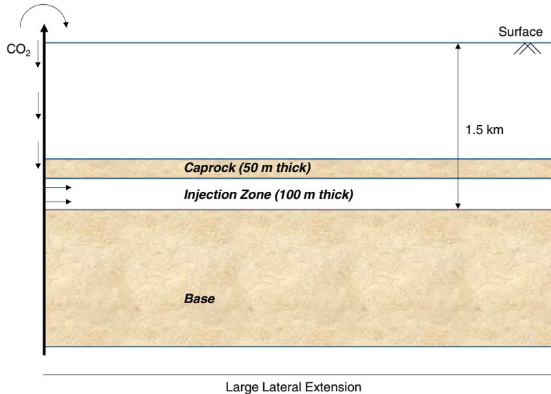
Fig. 1. Hypothetical test model for CO<sub>2</sub> injection and shear slip ( $\nu=0.25$  and  $\alpha=1$ ; original model from Rutqvist et al. [22]).
