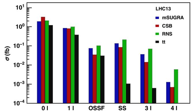
FIG. 4 (color online). Cross section after cuts from gluino pair production for the three SUSY benchmark models and from  $t\bar{t}$  background. For the 0 and  $1\ell$  signals, we take  $E_T > 500$  GeV while for the OSSF dilepton channel we take  $E_T > 400$  GeV. For the SS,  $3\ell$  and  $4\ell$  signals, we require  $E_T > 50$  GeV.
