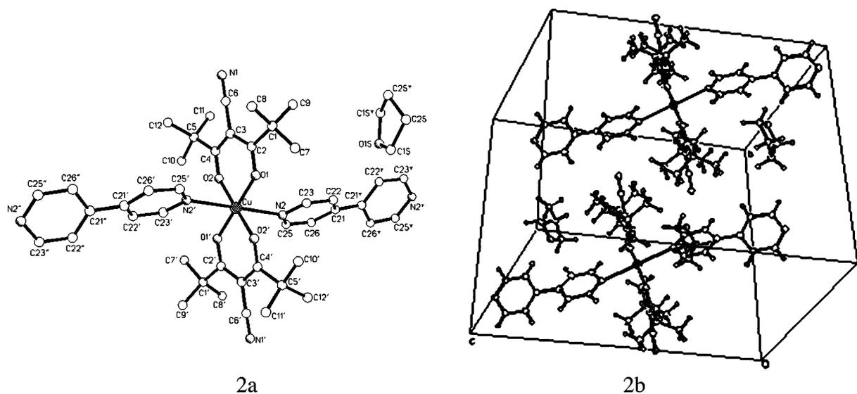
**Figure 2.** Single-crystal structure, **2a**, and unit cell packing diagram, **2b**, of  $\text{C}_{36}\text{H}_{48}\text{N}_4\text{O}_4\text{Cu}\cdot\text{C}_4\text{H}_8\text{O}$  (bis(4-cyano-2,2,6,6-tetramethyl-3,5-heptanedionato)copper(II) 4,4'-bipyridylethene-THF), i.e.,  $\text{Cu}(\text{CNdpm})_2\text{BPEA}$ .
