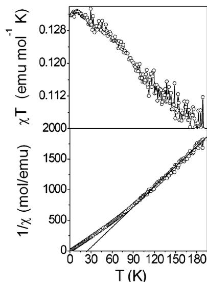
**Figure 5.** Ac susceptibility as a function of temperature for the Cu(CNdpm)<sub>2</sub>. The ac susceptibility measurements were done with  $H_{dc} = 0$  and  $H_{ac} = 3$  Oe. Susceptibility versus temperature (top) shows a negative slope, indicating ferromagnetic exchange. The inverse susceptibility (bottom) versus temperature indicates changes in the magnetic ordering at  $\sim 100$  K, where a positive Weiss temperature is determined.
