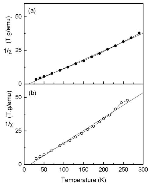
**Figure 4.** High-field inverse susceptibility, as a function of temperature, for  $\text{Cu}(\text{CNdp})_2$  (a) and  $\text{C}_{36}\text{H}_{48}\text{N}_4\text{O}_4\text{Cu}\cdot\text{C}_4\text{H}_8\text{O}$  (b). The inverse susceptibility data are derived from the temperature-dependent magnetization and have been fitted to a linear function to obtain the Curie constant (see text).
