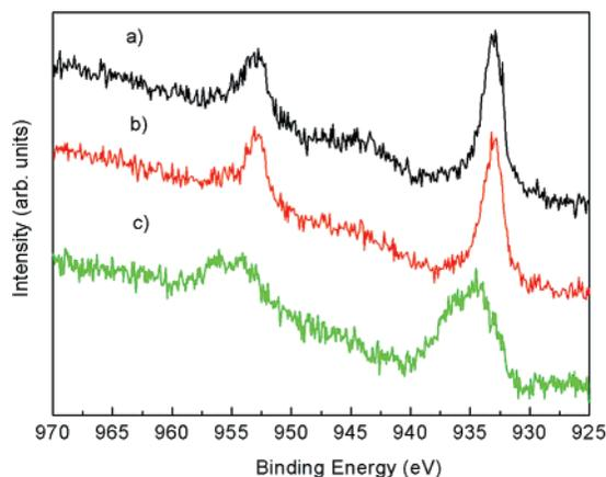
**Figure 9.** Cu  $2p_{1/2}$  and  $2p_{3/2}$  X-ray photoelectron spectroscopy for (a)  $C_{36}H_{46}N_4O_4Cu \cdot C_4H_8O$  and (b)  $Cu(CNdpm)_2$ , while (c) the decomposition of  $Cu(CNdpm)_2$ , due to electron irradiation at 50 eV, leads to a species with greater binding energy. All binding energies are referenced to the Fermi level.
