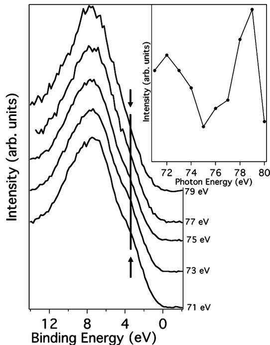
**Figure 8.** Photon energy dependence of thick Cu(CNdp) $_2$  film at 100 K. The valence band changes little with photon energy in the region 70–80 eV, although there are enhancements of the feature (the shoulder, indicated by the arrows) at about 5 eV binding energy, at photon energies in the vicinity of 79 eV, i.e., at the Cu 3p $_{1/2}$  core threshold. All photoelectrons are collected along the surface normal (normal emission).
