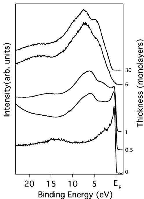
**Figure 6.** Coverage dependence of Cu(CNdpm)<sub>2</sub> adsorbed on an epitaxial Co(111) film at 100 K. The valence band development in photoemission of the Cu(CNdpm)<sub>2</sub>, with increasing molecular film thickness, on a 20 Å of Co(111) epitaxial film grown on a Cu(111) is shown for a photon energy of 61.5 eV. All photoelectrons are collected along the surface normal (normal emission). The estimated thickness of the Cu(CNdpm)<sub>2</sub> films are also indicated.
