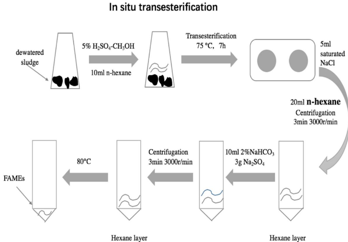
**Figure 4.** Biodiesel production process for secondary sludge<sup>2</sup>
