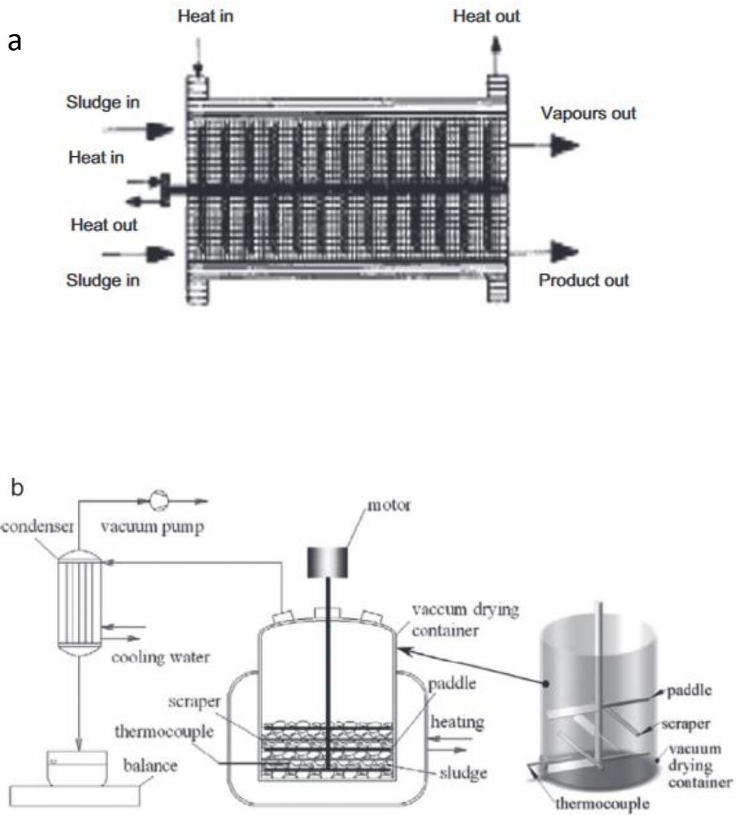
**Figure 2.** Different types of conductive dryers. a) disc dryer
