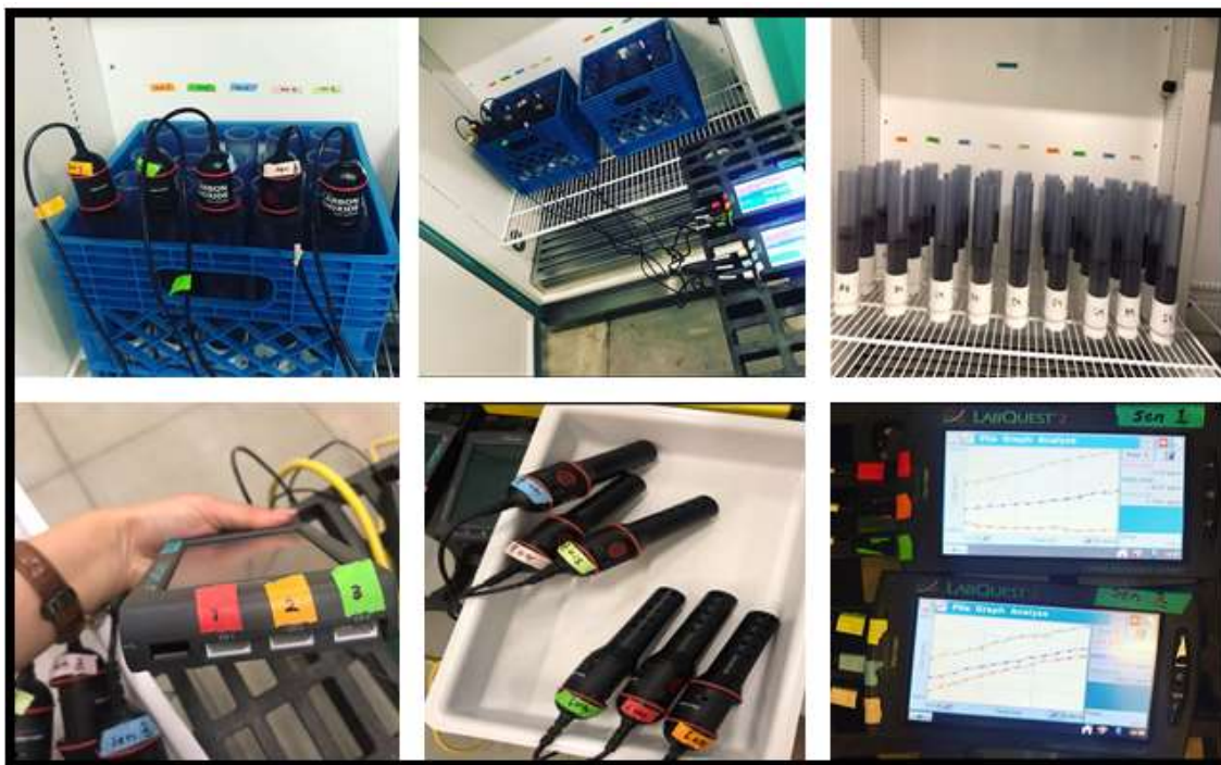
Figure 3-1. Vernier CO 2 Gas Sensor was placed inside each cylinder's headspace to measure CO 2 emissions in (mgL -1 ) of each treatment over time.
