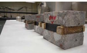
Figure 5. Concrete Blocks with Spacer Strips
