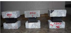
Figure 4. Concrete Blocks after 100% Extension — Visual Inspection
