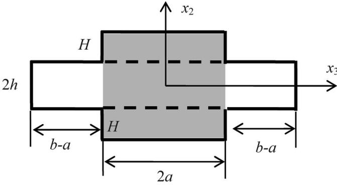
Fig. 1. A mesa resonator of AT-cut quartz.
