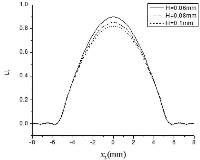
Fig. 5. Effect of  $H$  on the first mode.TABLE I. NUMBER OF TRAPPED MODES VERSUS  $a$ .
