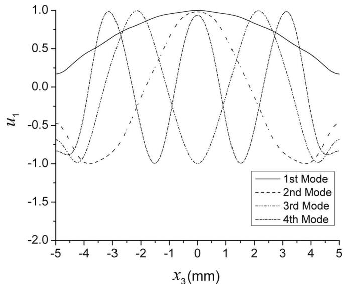
Fig. 3.  $u_1$  versus  $x_3$  at  $x_2 = h$  for the four lowest modes.
