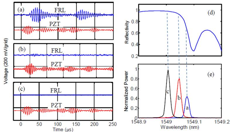
Fig. 5. (a-c) Responses from the FRL sensor system and the PZT sensor system to a ultrasonic pulse when the lasing wavelength was tuned to different positions on the slope of the FBG reflection spectrum (for clarity, the signals from the PZT are normalized and shifted in the vertical axis); (d) the FBG reflection spectrum; and (e) the lasing wavelengths corresponding to (a-c) and relative to the FBG spectrum shown in (d).
