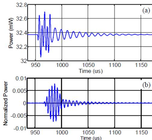
Fig. 3. Simulated sensor response to a 5-cycle 200 kHz ultrasonic pulse: (a) signal before the digital BPF and (b) signal after the digital BPF.
