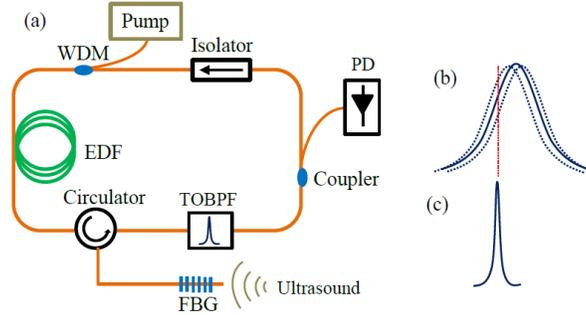
Fig. 1. Schematic of (a) the proposed FRL ultrasonic sensor system; (b) the reflection spectrum of the sensing FBG and the effect of the ultrasonic signal on the spectrum; and (c) the transmission spectrum of the TOBPF.
