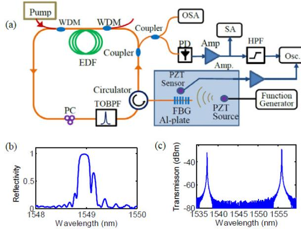
Fig. 4. (a) Schematic of the experiment set up; (b) normalized reflection spectrum of the sensing FBG calculated from the measured transmission spectrum; and (c) measured transmission spectrum of the TOBPF. PC: Polarization controller; Osc.: Oscilloscope.
