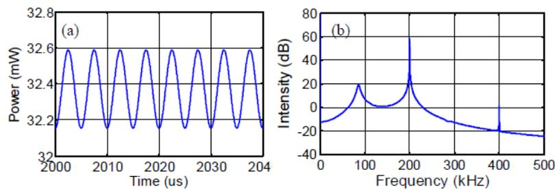
Fig. 2. (a) Simulated sensor response to a 200 kHz continuous sinusoidal ultrasonic signal; (b) spectrum of the sensor response.
