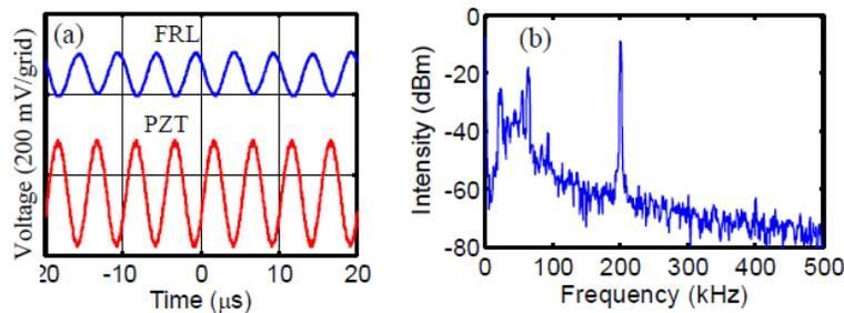
Fig. 6. (a) Signals recorded by the oscilloscope from the FRL sensor system and the PZT sensor system when the sensors were applied to a 200 kHz continuous sinusoidal ultrasonic signal (for clarity, the signal from the PZT is normalized and shifted in the vertical axis) and (b) Spectrum recorded by the SA for the amplified RFL output signal.
