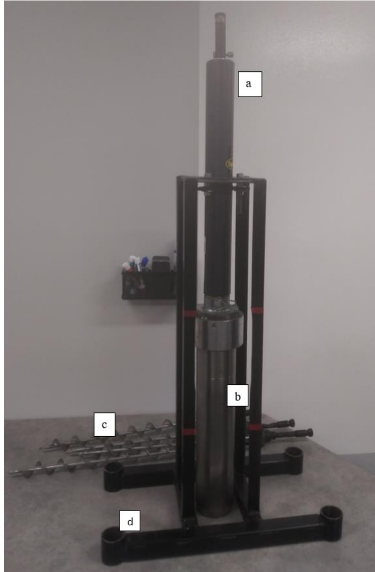
Figure 2. The second soil probe built to take 30 cm soil cores from golf course putting greens. This soil probe used a hydraulic truck jack (a) to push the soil core into the ground. Also pictured is the stainless steel sleeve (b) in position for collecting a sample, the four augers (c) needed to keep the soil probe in place during sampling, and the anchor spots where augers are inserted with a hand-held drill (d).
