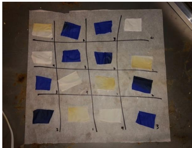
Figure 1: The image shows the latin square arrangements, with squares 1 and 4 with latex gloves, 2 and 3 with nitrile gloves. Squares 1 and 2 were treated with 24 hours of UV light, and are visibly discolored.
