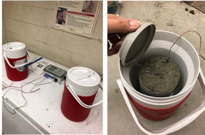
Figure 3-6. Maturity meter test setup
