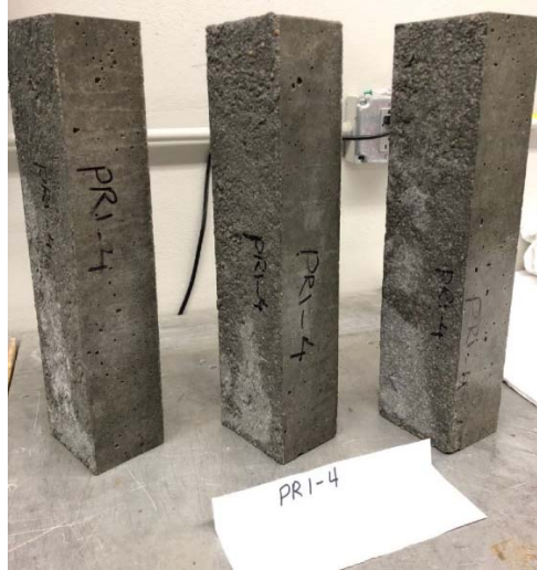
Figure 3-10 Wet/Dry specimens after 28 days of curing
