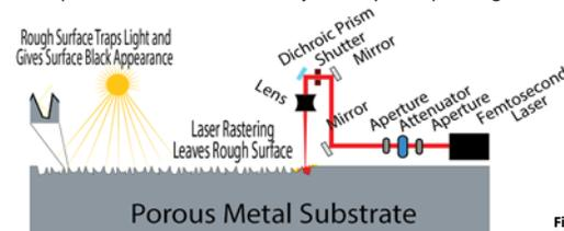
Figure 7. Schematic of femtosecond laser processing and light trapping geometry
