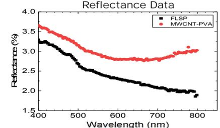
Figure 10. Graph of light reflectance percentages for spray coated and laser processed solar absorption layers across different wavelengths
