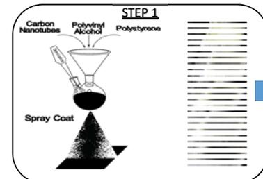
Figure 4. Schematic of synthesizing steps for spray coating a PVDF film with MWCNT solution
