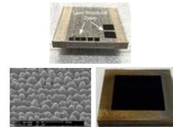
Figure 8. SEM image of rastered metal surface (Left).<sup>[2]</sup> Image of metal substrate with laser processed zones (Top).<sup>[2]</sup> Image of metal substrate with entire surface laser processed (Right).<sup>[2]</sup>
