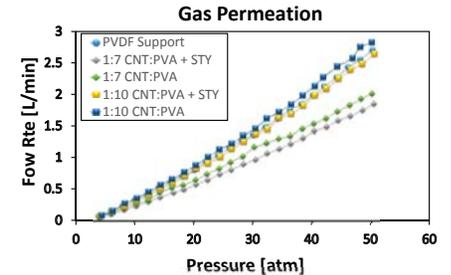
Figure 9. Graph of nitrogen flow rates through varying composite membrane ratios at different pressures
