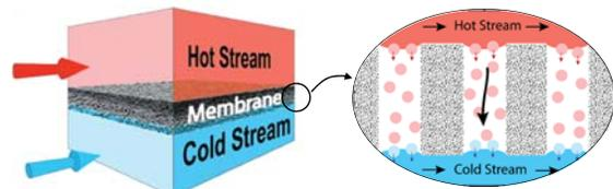
Figure 1. Schematic of MD process, where a hydrophobic membrane acts as a physical barrier between hot and cold streams but allows water vapor to diffuse through its pore channels.
