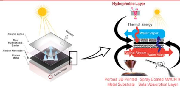
Figure 3. Three-dimensional (3D)<sup>[1]</sup> and two-dimensional (2D) schematics of a solar-integrated device. The composite membrane consists of four parts: a Fresnel lens, a thin porous hydrophobic barrier, a solar absorption layer, and a porous metal substrate produced from additive manufacturing methods.
