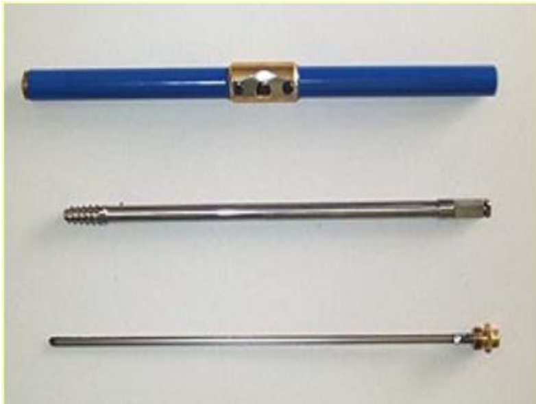
Figure 1. Dismantled increment borer showing all parts (Cardwell, 2004).
