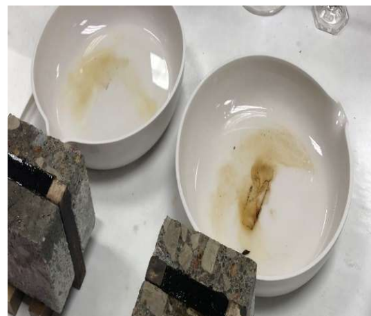
Figure 9 - The Product 2, 1-min (left) and 5-min (right) tests show dissolution.
