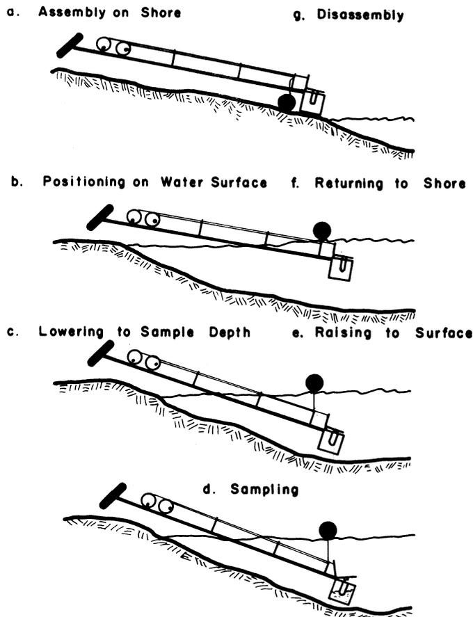
FIG. 1 Pond water sampler operation scheme.
