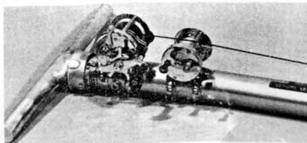
FIG. 2 Operator end of sampling device. The T-handle and reels provide a convenient control point. One reel contains the cord to the float; the other reel contains the cord to the sampler head.
