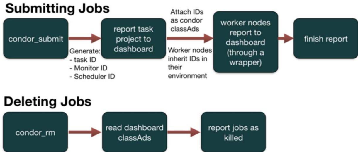
**Figure 5.** Diagram of the CMS Dashboard integration.
