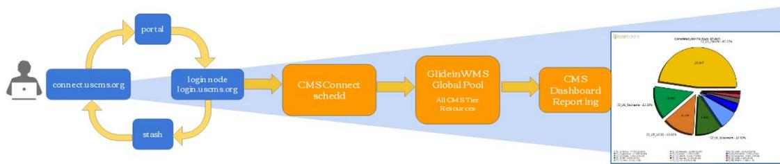
**Figure 3.** CMS Connect main components.
