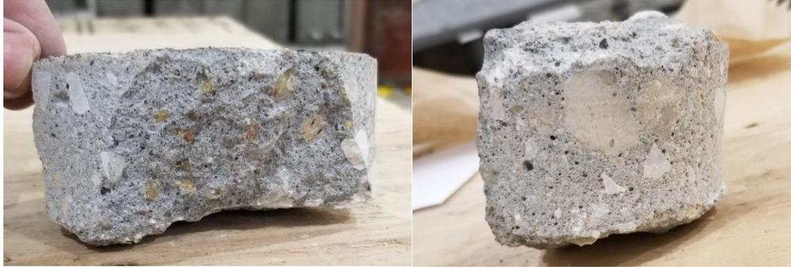
**Figure 30.** Extracted cores from the concrete specimen
