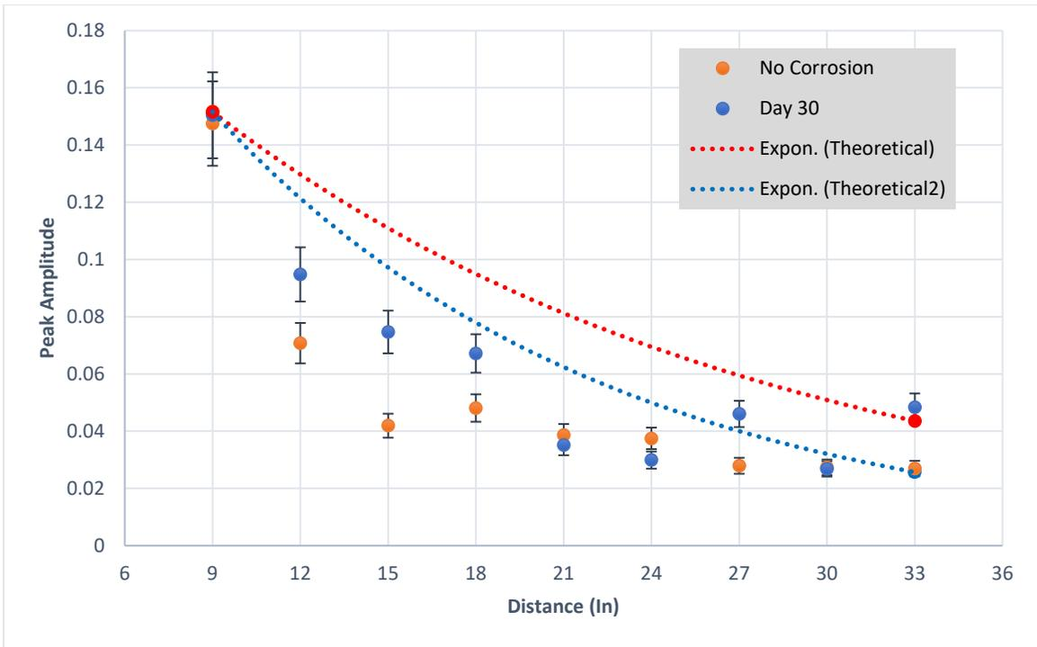
Figure 21. Specimen A-UGWL readings for Day 0 and Day 30
