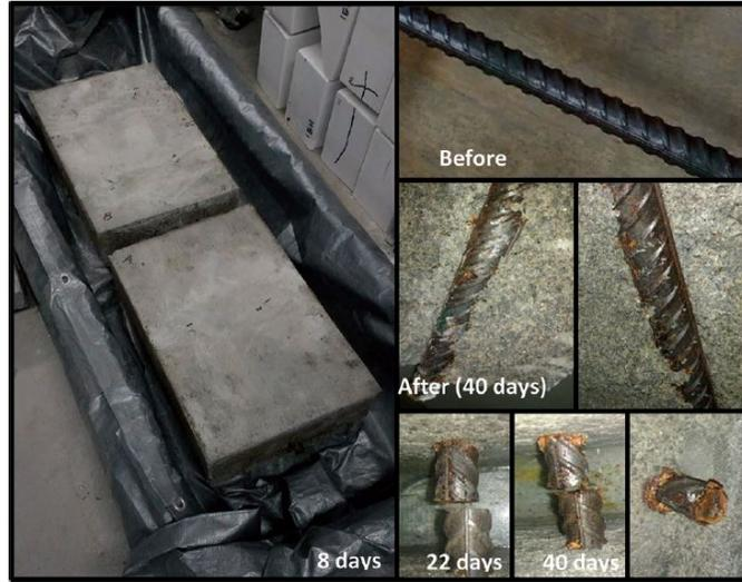
**Figure 1.** Corrosion specimens (Garcia et al., 2019)
