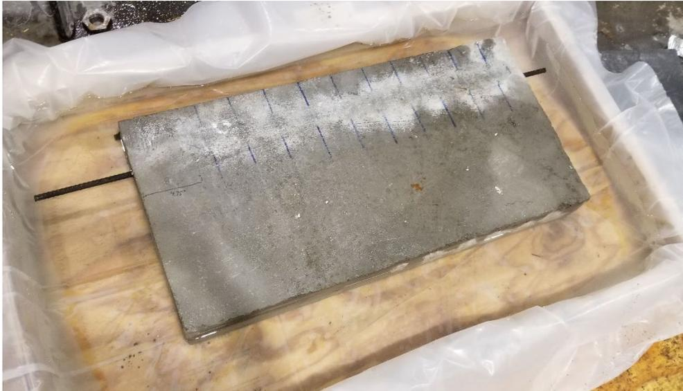
**Figure 16.** Test specimen submerged inside 10% NaCl solution
