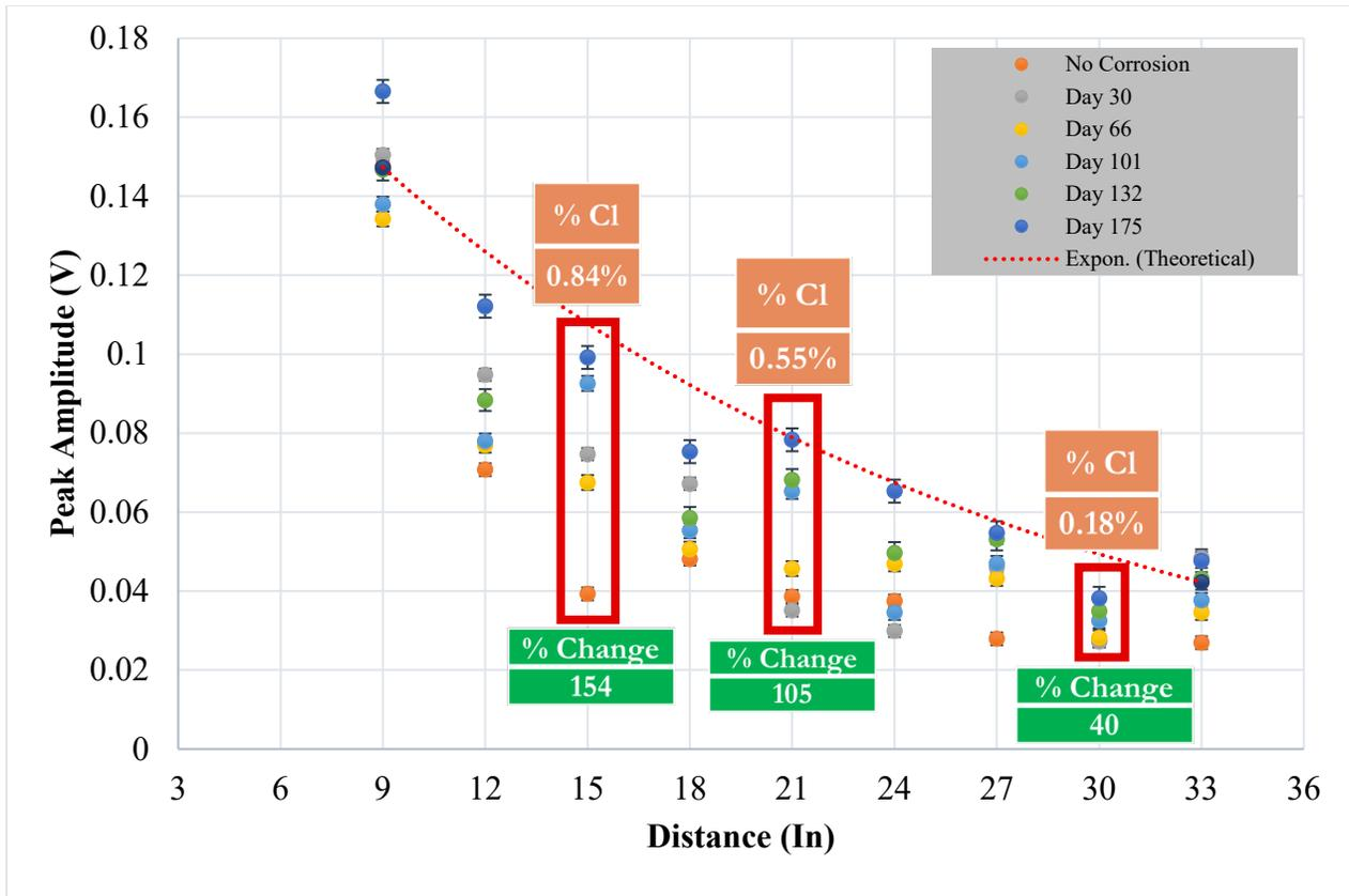
**Figure 33.** Correlation between UGWL data and chloride content
