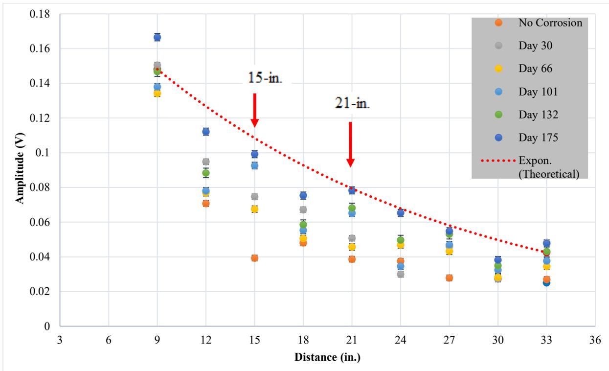
Figure 22. Specimen A-UGWL readings combined plot for 0-175 days
