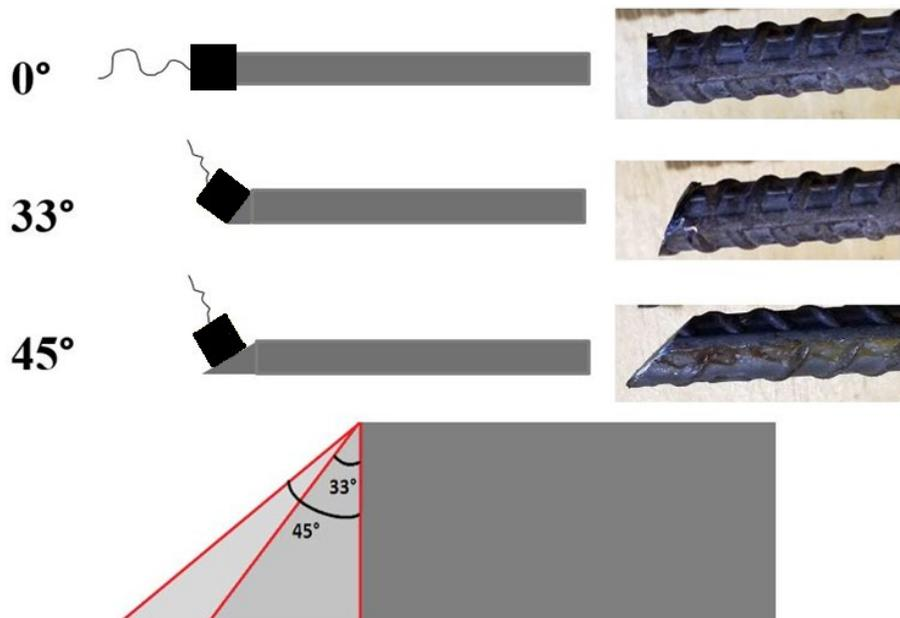
**Figure 4.** Bar end angles used in Specimen Set 1
