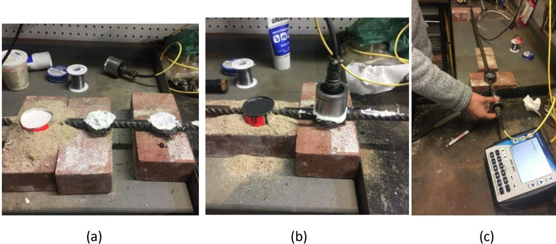
**Figure 34.** Attachment options: (a) Direct energy transmission; (b) Transducer coupled to solder pad and epoxy pad curing in sheet metal form; and (c) Solder and epoxy pads fully cured. Gypsum cement poured into sheet metal form
