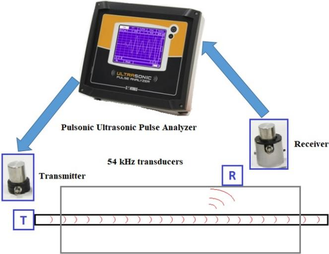
**Figure 5.** Experimental set-up for UGWL testing procedure
