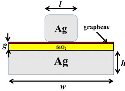
Fig. 1. The cross-section profile of the periodic film-coupled nanowires loaded with graphene.
