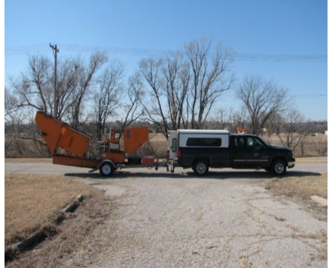
Figure 1 - Falling Weight Deflectometer (FWD) measures modulus via deflection with 7 sensors and machine-dropped weights.
