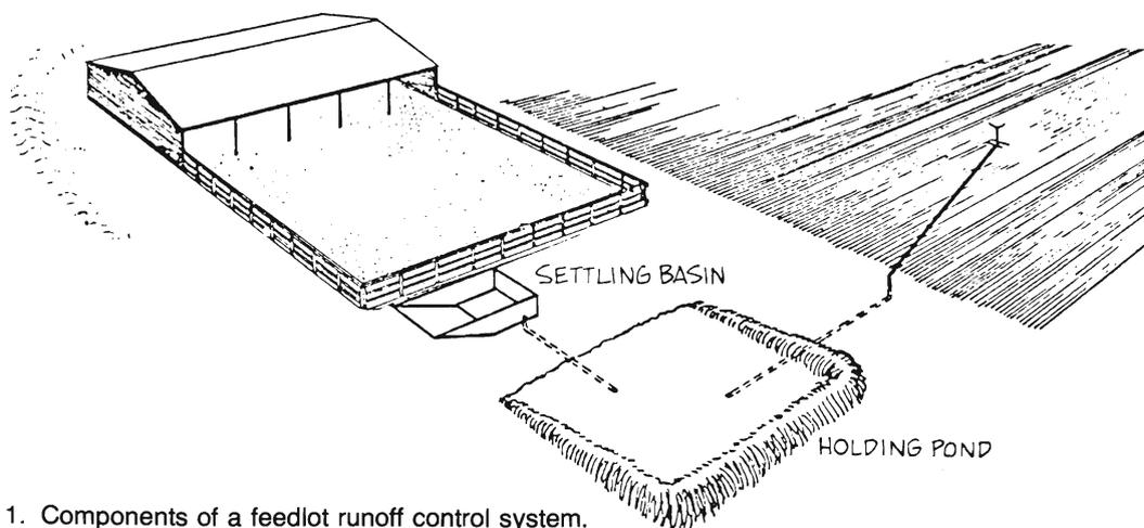
Figure 1. Components of a feedlot runoff control system.
