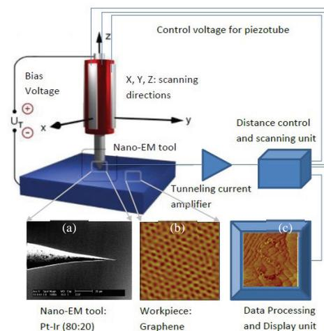
Fig. 1. Schematic representation of the nano-EM setup; (a) SEM image of atomically sharp Pt-Ir (80:20) tip, (b) atomic resolution the STM image of the graphene surface, and (c) machining of letter "S" on graphene as shown in the display unit after machining by nano-EM.
