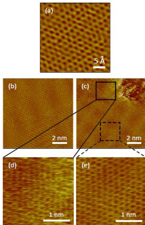
Fig. 2. (a) Atomic resolution STM image of graphene ( $3 \text{ nm} \times 3 \text{ nm}$ , 200 mV, 1 nA), (b) Current image (constant-height) of  $10 \text{ nm} \times 10 \text{ nm}$  graphene surface before machining (200 mV, 1 nA), (c) Current image of the same  $10 \text{ nm} \times 10 \text{ nm}$  graphene surface after machining (at 2600 mV, 1 nA, 3 sec), (d) Magnified image taken adjacent to the machined nano-hole, (e) Magnified image taken from un-machined area.
