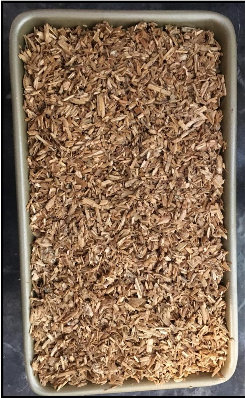
*Figure 3: Mycelium-hemp product - post oven baking*
