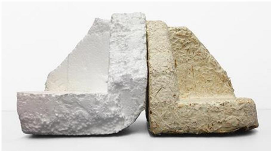
*Figure 2: Polystyrene packaging side by side to mycelium hemp packaging (Rosenbaum 2016)*
