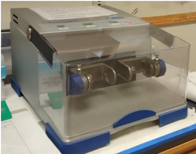
Figure 15: TissueLyser used in this study to break down leaf tissue samples.
