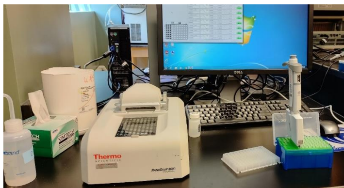
Figure 17: Spectrophotometer used in this study to determine quality of DNA samples collected.
