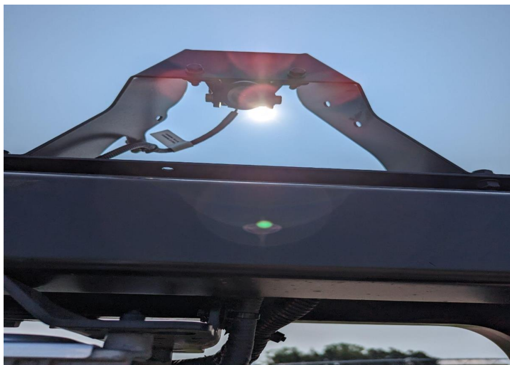
Figure 3. One of 36 cameras attached to boom of John Deere See and Spray used in spot spray trials conducted near Mead, NE in 2023.
