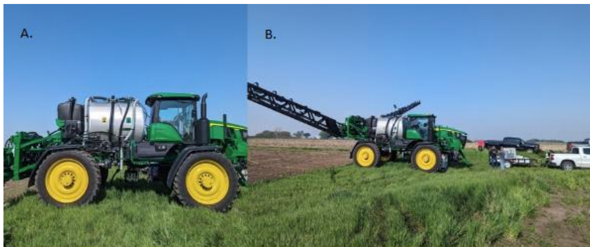
Figure 1: John Deere's precision sprayer with a.) dual tank system; b) unfolded (37 m wide boom) before application in field experiment conducted in soybean near Clay Center, NE in 2023.
