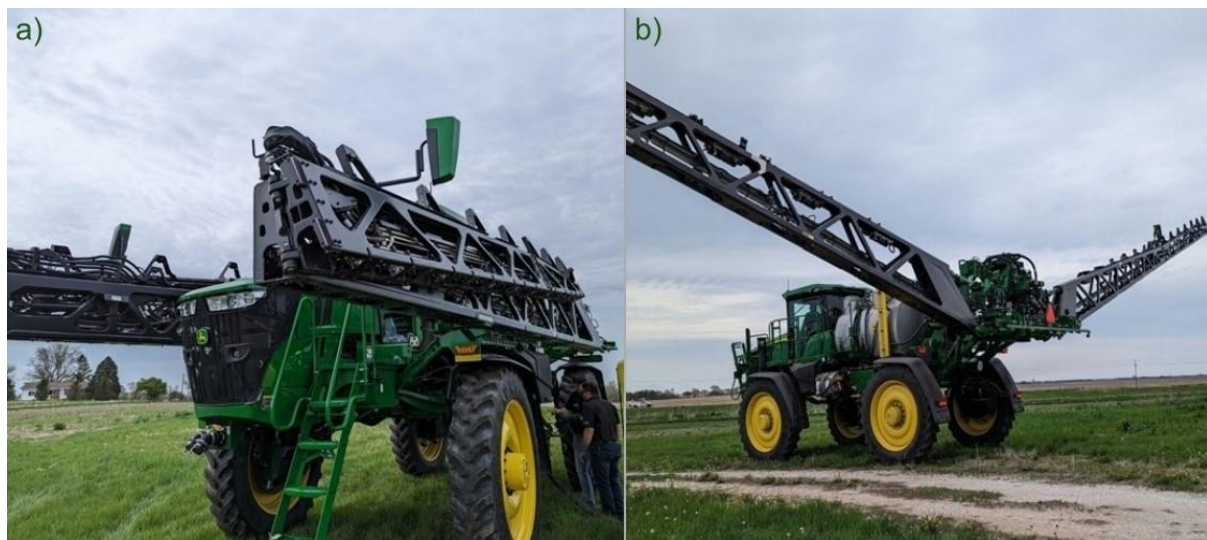
Figure 2. John Deere' See and Spray machine with boom a) folded and b) unfolded (37 m wide boom) before A application in spot spray trial conducted in soybean near Mead, NE in 2023.
