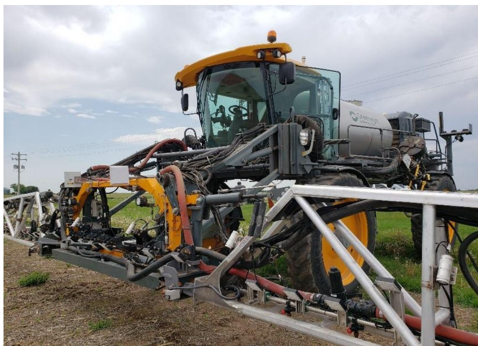
Figure 1. Greeneye technology machine used in spot spray trial conducted in corn near Clay Center, NE in 2022. This system can be retrofitted on compatible sprayers.
