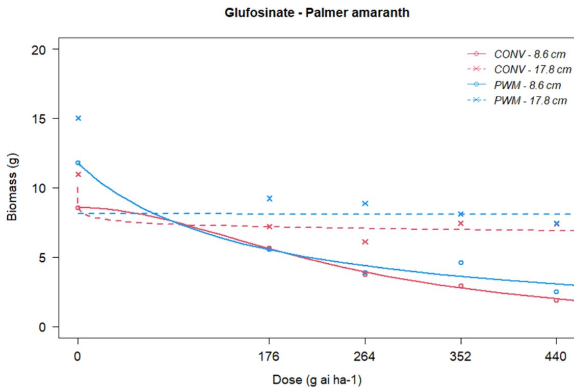
**Figure 3-2.** biomass reduction of palmer amaranth over the dose range applied of glufosinate. Abbreviations: CONV – 8.6 cm, variable dose with fixed volume method sprayed on 8.6 cm plants; CONV – 17.8 cm, variable dose with fixed volume method sprayed on 17.8 cm plants; PWM – 8.6 cm, variable dose with PWM method sprayed on 8.6 cm plants; PWM – 17.8 cm, variable dose with PWM method sprayed on 17.8 cm plants.
