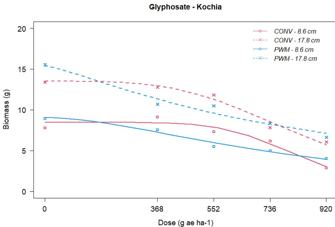
**Figure 3-4.** biomass reduction of kochia over the dose range applied of glyphosate. Abbreviations: CONV – 8.6 cm, variable dose with fixed volume method sprayed on 8.6 cm plants; CONV – 17.8 cm, variable dose with fixed volume method sprayed on 17.8 cm plants; PWM – 8.6 cm, variable dose with PWM method sprayed on 8.6 cm plants; PWM – 17.8 cm, variable dose with PWM method sprayed on 17.8 cm plants.
