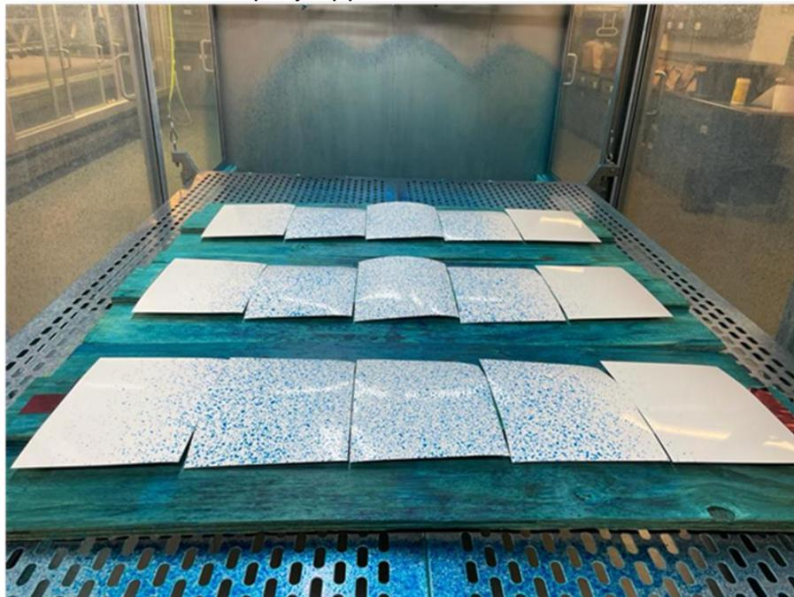
figure 2. layout of kromekote cards for coverage and spray pattern analysis
