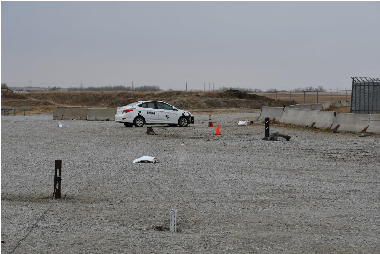
Figure 51. Vehicle Final Position and Trajectory Marks, Test No. NMB-1
