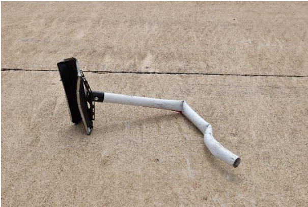
Figure 11. TxDOT Large Mailbox on Type 4 Support - Test No. 469689-1-1, Test Results
