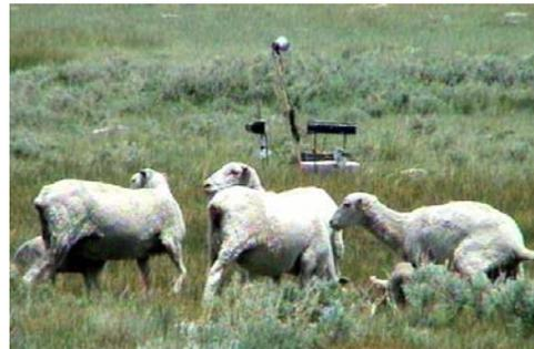
In their current experimental form, our systems would likely be most practical for use where sheep are kept in fenced pastures and bedded in the same locations each night. The devices are not quickly installed and bulky to move, partially because they require three or four 12-V deep-cycle batteries, each weighing 27 kg. Daily attention was required to ensure adequate air pressure, because > 65 p.s.i. was needed to erect the pop-up scarecrow.
