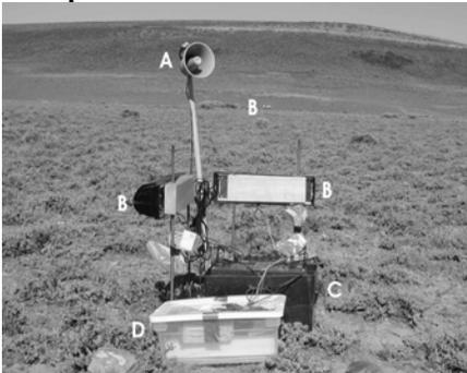
**Figure 2. Animal-activated acoustic frightening device with added pop-up scarecrow and a strobe light evaluated in the protection of domestic sheep from coyote predation, Wyoming, 2002. A. All-weather speaker, B. infrared sensors, C. 12-V batteries, D. CD electronics in protective case, E. high-pressure air storage tank, F. scarecrow, and G. strobe light, .**
