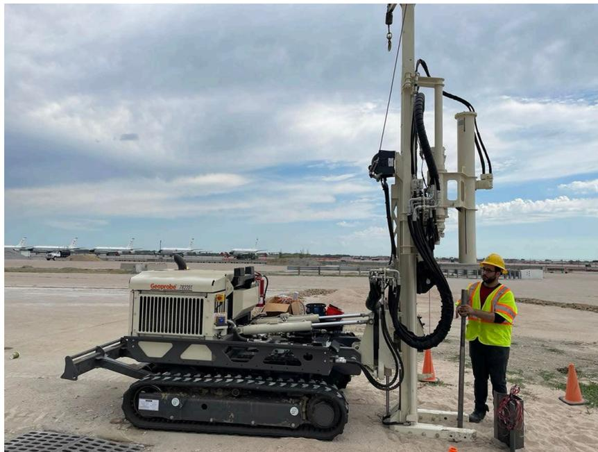
Figure 4.11 SPT test conducted by the research team.
