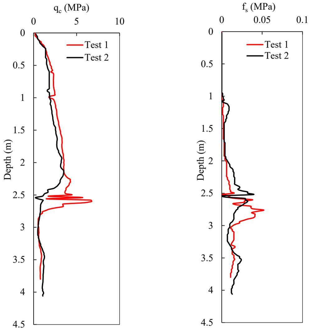
Figure 4.14 The tip resistance  $q_c$ , and skin resistance  $f_s$  (left to right) obtained from CPT tests.
