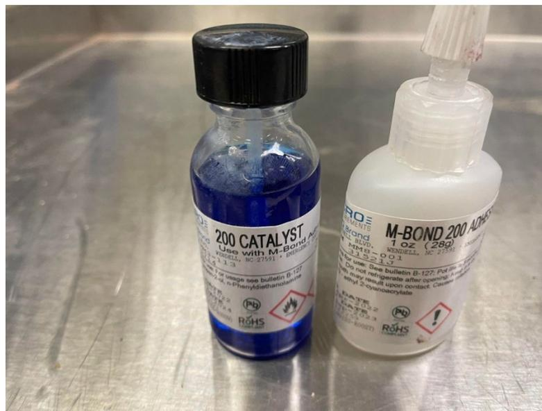
Figure 4.17 Cleaning liquid and adhesive used for resistive strain gauge installation (from Micro-Measurements VPG).
