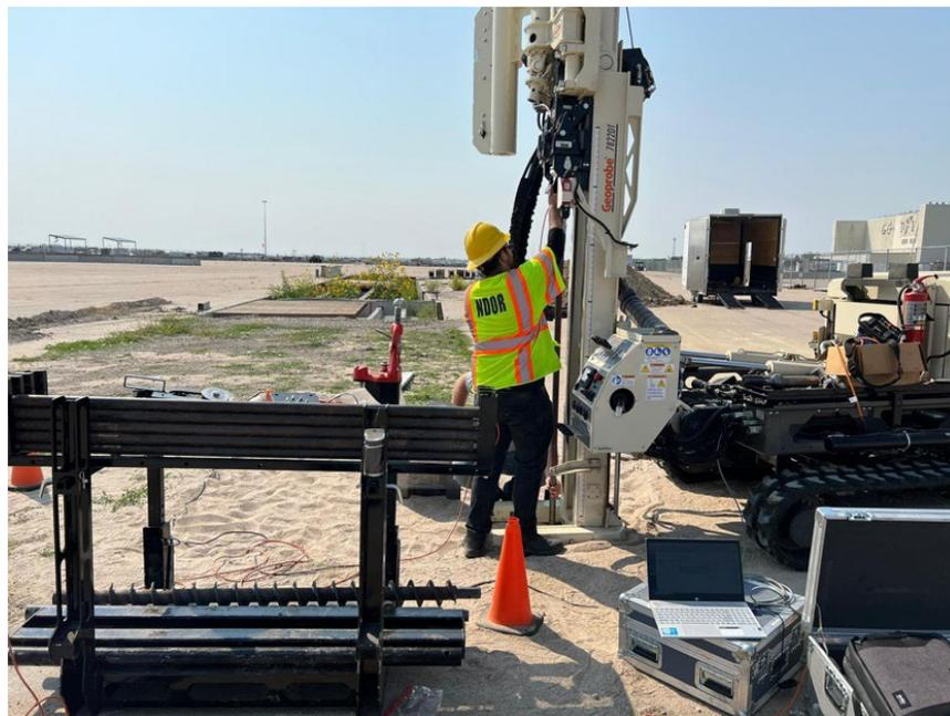
Figure 4.13 CPT test conducted by the research team.
