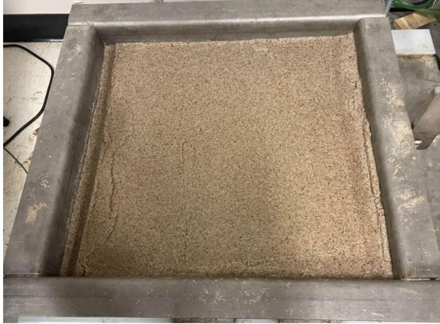
Figure 3.6 Fill sand in the shear box.
