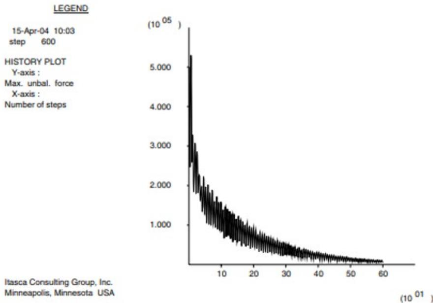
Figure 5.1 An example of maximum unbalanced force for the problem of sudden end-load application to a column (Itasca Consulting Group, 2019).
