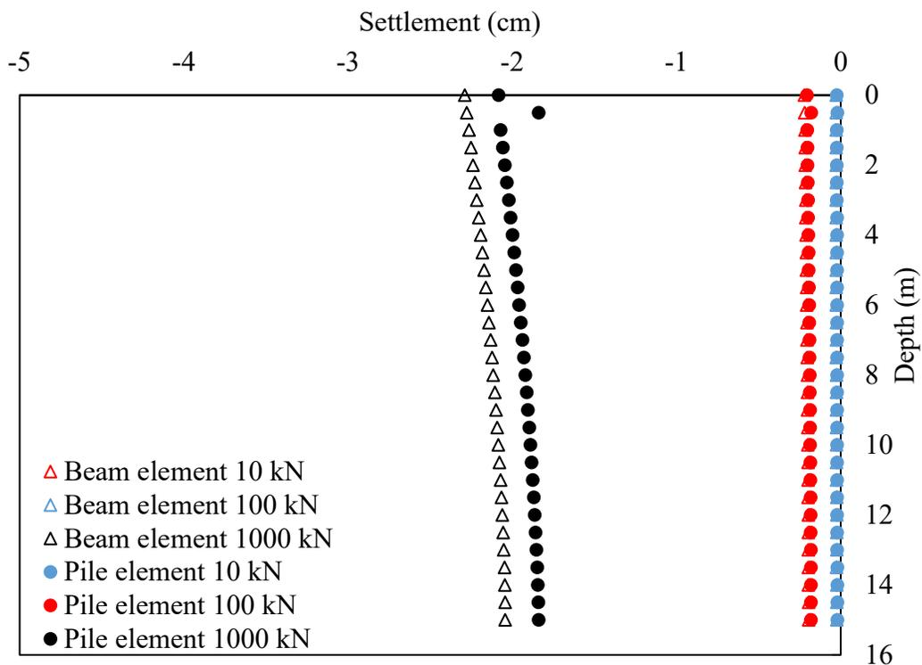
Figure 5.5 The comparison of vertical settlements from the models that use either the beam element or pile element. Three level of axial loads (10 kN, 100 kN, and 1000 kN) is applied to the numerical simulation. Note: 1 inch = 2.54 cm.
