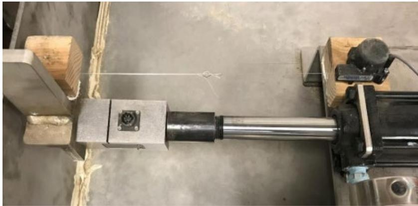
Figure 3.9 The horizontal LVDT.
