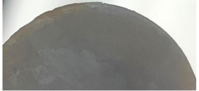
*Figure 2: Pellet with small grains that does not allow the as much of the light from the back-side illumination through. Density is 94% of the theoretical maximum.*
