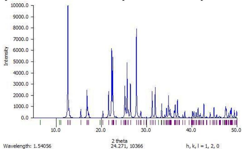
Figure 10: This is the simulated spectra for orthorhombic DIPAB
