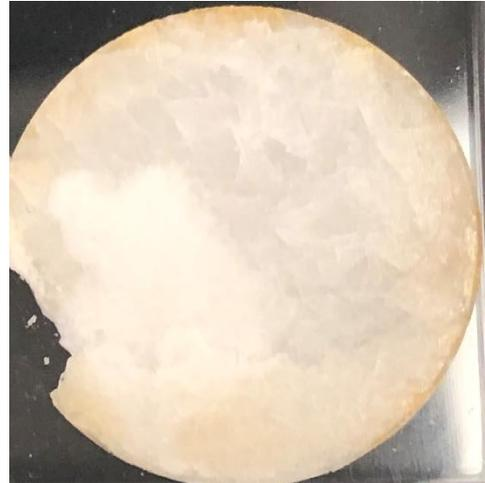
Figure 5: This is an example of a pellet which only has surface oxidation around the edges of the pellet. Often times this is the best case for a pellet.
