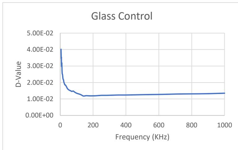
Figure 1: The graph of the dissipation factor vs frequency for a glass standard
