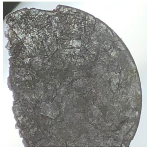
*Figure 3: Pellet shown with illumination on the back side contains larger crystal grains that allow more light to be transmitted by the pellet. 85% of the theoretical maximum density.*
