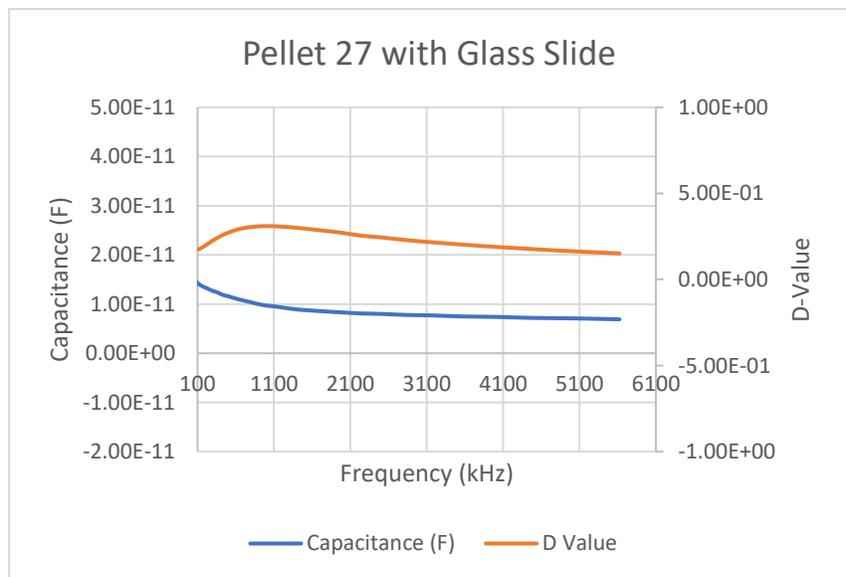
Figure 6: This is the capacitance and D-Value data for both the ceramic pellet and a glass slide. It shows that the measurements read are accurate as it is within 7 pF of the expected 18pF capacitance for the system, while the D-value is relatively low.
