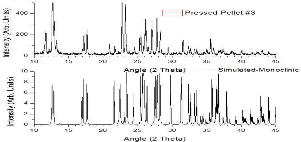
Figure 9: This image shows the spectrum from a pressed pellet that had been annealed. It is lacking the peak at 16 used for the identification of the orthorhombic phase. This combined with the fit of the other peaks indicates that this pellet is monoclinic.
