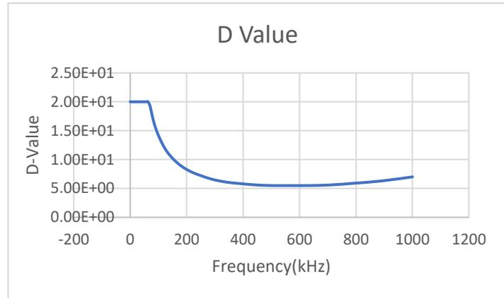
Figure 7: Here shows a measured D-value not being inversely proportional to frequency. The value is also large and indicates that the measured capacitance is not accurate.
